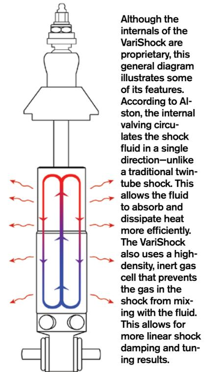
Although the internals of the VariShock are proprietary, this general diagram illustrates some of its features. According to Alston, the internal valving circulates the shock fluid in a single direction—unlike a traditional twin-tube shock. This allows the fluid to absorb and dissipate heat more efficiently. The VariShock also uses a high-density, inert gas cell that prevents the gas in the shock from mixing with the fluid. This allows for more linear shock damping and tuning results.
