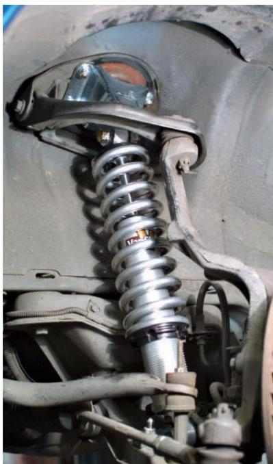
We have to admit that we sort of dig this bolt-on coilover conversion for fourth-gen Camaros. The bracket at the top attaches to the A-arm mount like a stock setup. According to Alston, the "extra-long" shock allows for extensive choices of ride height, spring rate, and shock valving.
