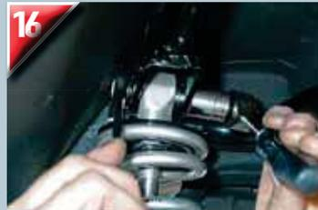
Coil-over VariShocks are installed next, top first. This is a tight spot, so expect it to be challenging.
