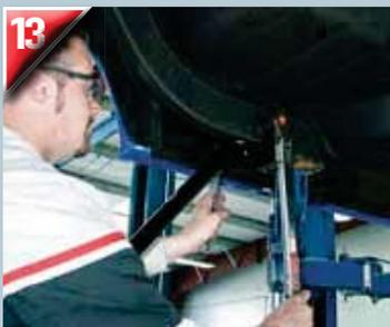
Control arm (trailing arm) fasteners are torqued to 60 lb-ft. Make sure the grease jerks are accessible before tightening.
