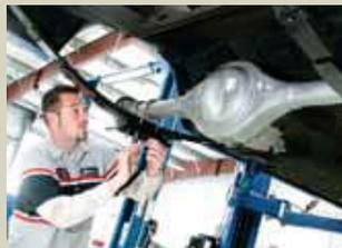
As shown in a previous article, Currie's good-looking 9-Plus housing, filled with 9-Plus 3.89:1 limited-slip locking gears and 28-spline axles, is centered on the Grab-A-Trak five-leaf, mid-eye springs.
