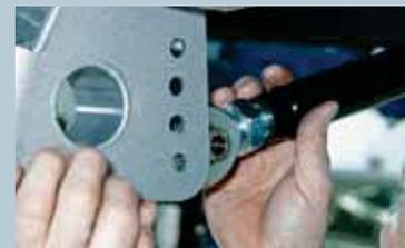
Lower control arms should be 21 inches center to center. Again, expect some variation. Position the lower arms as close to the vehicle ride height location as possible. TCP provides three hole positions in the axle mount. The lower arms control alignment.
