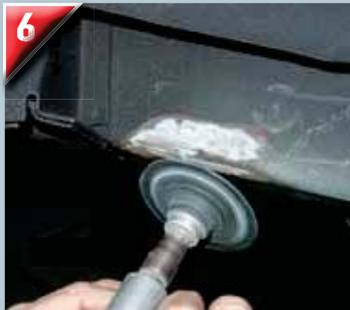
Remove the paint and undercoat where you intend to weld. The Restomod Shop suggests welding in addition to bolting for a secure installation.
