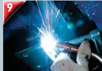
With the subframe positioned and clamped, Richard strikes an arc and welds a smooth bead along the bracket.
