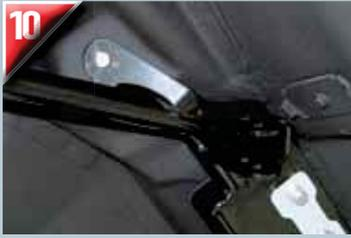
The subframe also attaches at the original shock mounts and rebound bumper location. Shock location fasteners are torqued to 40 lb-ft. Rebound bumper fasteners are torqued to 20 lb-ft. The rebound bumper is also known as a pinion snubber.
