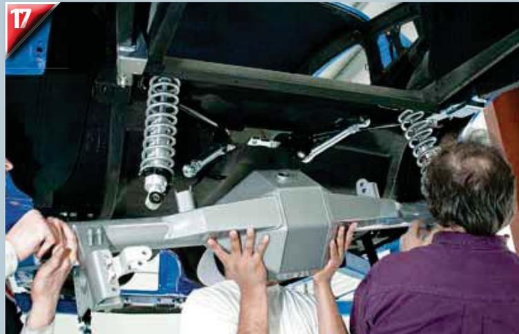
Chris Alston's FAB-9 housing is attached at the shocks and lower control arms. The FAB-9 makes our TCP package complete and ready for anything.
