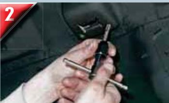
The first step for the g-Link system installation is chassis prep, which isn't saying much. Chase bolt-hole threads to ensure smooth engagement. Here, we have removed the rebound bumper, which is one of the attachment points.
