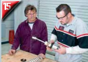
Coil-over shock assembly is next. The lower spring mounts are screwed on before positioning the springs, followed by the spring locks. Richard will have to adjust spring pressure (which affects ride height) before adjusting the Quick Set Two-Valve system.
