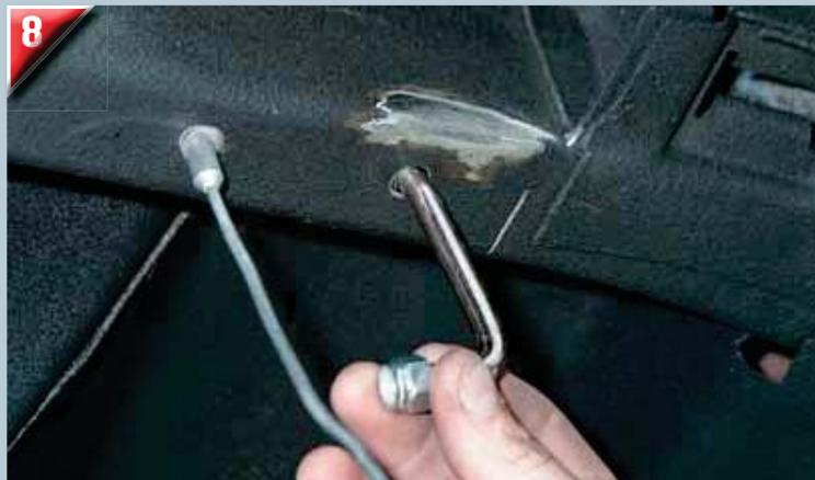
This is how to install the 1/2-20x5x3-inch U-bolt, which attaches the subframe to the frame rail. Richard uses a magnet to guide the U-bolt. Once in place, we're ready for subframe installation. Be careful never to lose this U-bolt inside the frame rail. Position the subframe and install flat washers and locknuts. Locknuts are torqued to 30 lb-ft.
