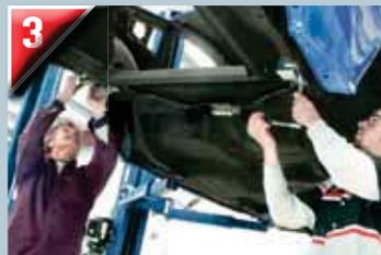
Once the g-Link subframe is assembled as a subassembly, we're ready for a mock-up fit. Use your Mustang's attachment points and a tape measure to ensure a perfect fit.
