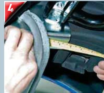
With the subframe positioned and C-clamped in place, get your measurements. There should be exactly 10 inches from the trailing edge of the subframe bracket to the leading edge of the rebound bumper bracket. If measuring from the leading edge of the rebound bumper bracket to the leading edge of the subframe bracket, it should be 4-1/4 inches.
