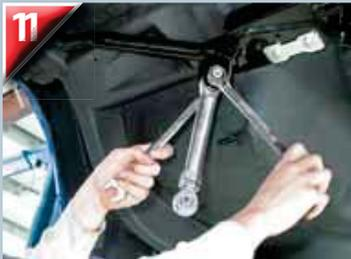
Trailing arms are next, which begins with simple tightening followed by the use of a torque wrench. You can install these trailing arms either way, but we suggest locating the Heim joint where access is easiest at the axle housing. This enables you to adjust the pinion angle and rearend alignment.
