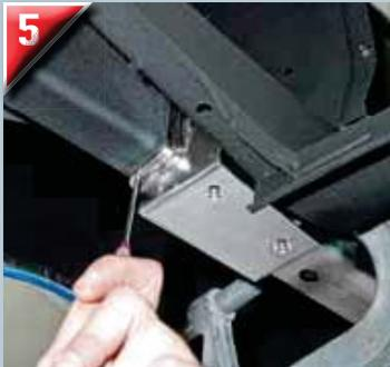
When you have committed to a location and are positive about measurements, scribe the holes and edges as shown. Be absolutely certain about location before drilling and welding.
