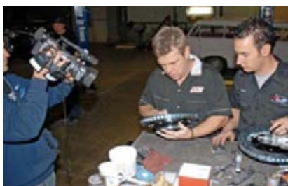
With the camera's rolling, Woods and Project Director Bret Maxwell focus (excuse the pun,) on installing the 11-3/4-inch vented directional rotor, Wilwood front disc brakes. First the mounting holes are all chased using the proper size tap.
