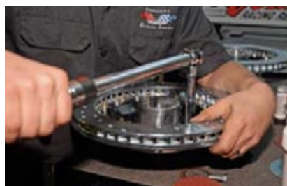
Setup begins with the billet hub(s) being fitted to the backside of the rotor. The provided 12-point bolts measure 2-1/4-inches in length, and should be final torqued in sequence according to the Chassisworks Instruction Manual.
