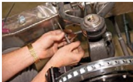
Next, our installers drill and tap the side of the Chassisworks frame for two 10-32-inch threaded holes. These holes will position the brake line tab 2-inches below the top of the frame and 2-1/2-inches ahead of the weld on the front cross member. Once these holes have been made, the accompanying stainless-steel brake line brackets are installed using the provided 10-32 x 3/8-inch button head bolts.
