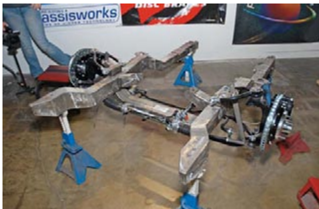
Shown is the 90% completed Alston Chassisworks front frame.
