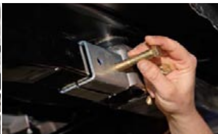
With sub frame connectors fitted in place, the mounting holes are drilled, and the combination 3/8-inch and 7-20 x 3-inch bolts are bolted into place.
