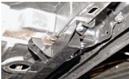
With sub frame connectors fitted in place, the mounting holes are drilled, and the combination 3/8-inch and 7-20 x 3-inch bolts are bolted into place.
