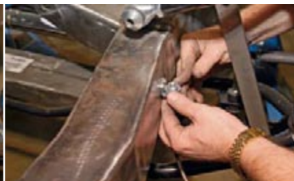
Next, our installers drill and tap the side of the Chassisworks frame for two 10-32-inch threaded holes. These holes will position the brake line tab 2-inches below the top of the frame and 2-1/2-inches ahead of the weld on the front cross member. Once these holes have been made, the accompanying stainless-steel brake line brackets are installed using the provided 10-32 x 3/8-inch button head bolts.
