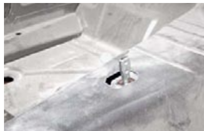
Next, Maxwell and company measure straight up from the shifter location of the TKO 600 transmission, and cut a "shifter slot" measuring approximately 1-1/2 x 3-inches in the center of the transmission tunnel.
