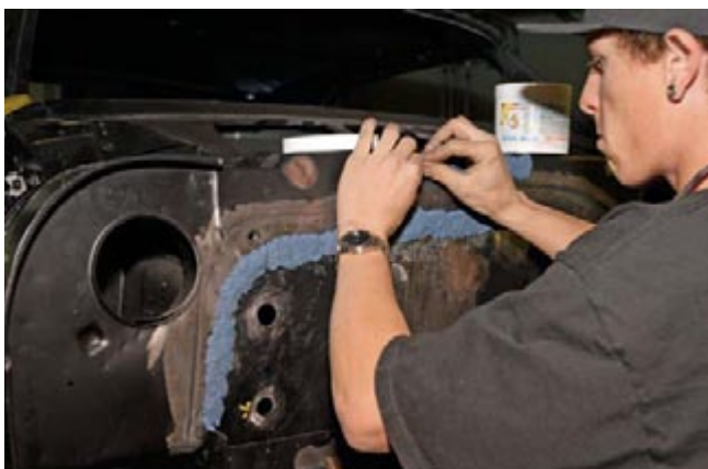
Other firewall modifications include seam-welding the entire circumference of the firewall using a special heat absorbing putty called "Cool Blue" which was applied to the larger areas to avoid warp-age.
