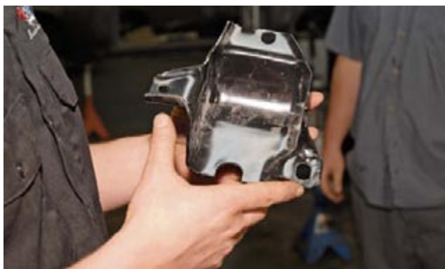
On the opposite end our crew installs the OE reproduction spring bucket for the Camaro rear leaf springs to "sit" in using the OE bolts provided.
