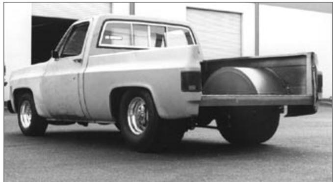
▲ The former beater awaits its successful test run - and an engine swap that will replace its tired small-block with a healthy rat motor. Matching 15x14- and 15x8-inch Weld Pro Star Truck wheels respectively rotate Mickey Thompson 33119.50- 15 LT and 255/60-15 tires.
