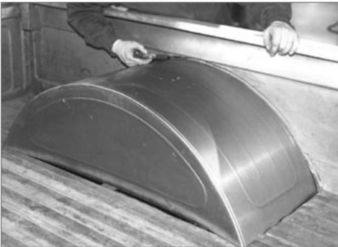
▲ Outer edge of heavy-gauge, factory assembled steel tub is marked to follow body contour, then trimmed and welded to both the wall and floor. (For Stepside trucks with wooden floors, Chassisworks provides angle strips that rivet to the tubs and screw into the floor.)
