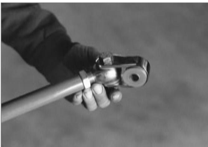
▲ Unique, double-clevis ends of Chassisworks' Pro Street locator eliminate suspension binding by allowing the locator to pivot in any direction.
