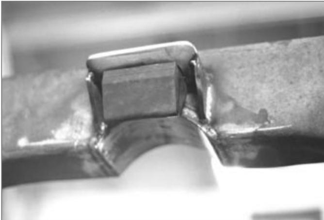
▲ Stock axle snubbers are relocated above each notch and welded directly to the frame.
