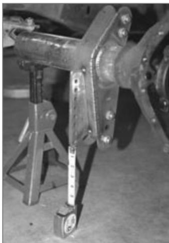
◀ After the bracket gussets are welded, shock mounts are positioned and tack-welded.
