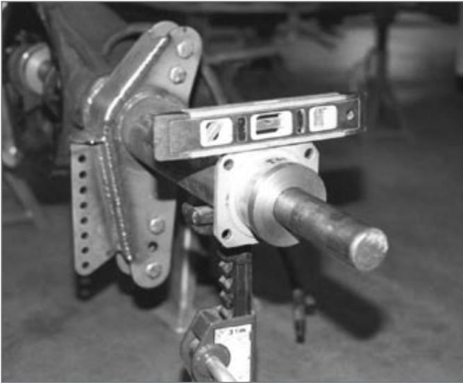
▲ Chassisworks' rearend-narrowing kit is used to precisely center housing-end mounting flanges for welding.
