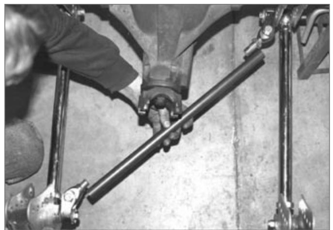
▲ With lower link bars installed, the track locator is cut to fit between two of Chassisworks' new double-clevis joints. Forward end of the tube welds on; the opposite end is threaded to accept a rod end.
