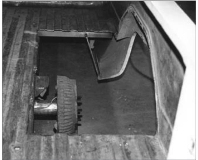
▲ Weld wheels and massive M/T tires were removed for fitting of new Chassisworks truck tubs. Floor cut follows the outside of the frame rail and is centered over the axle.
