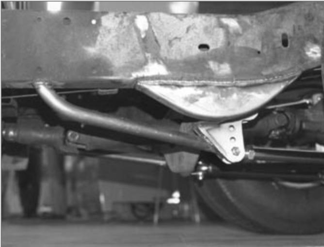
▲ Super-rigid suspension assembly Includes tubular bracing from the frame to the lower 4-link brackets, plus a small gusset plate between the top of each bracket and a stock crossmember (not visible).
