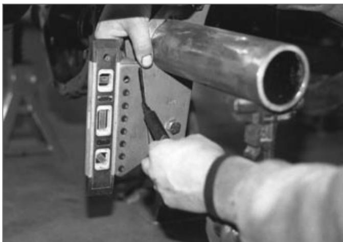
▲ Before gusset plates are welded to the 4-link brackets, each lower shock mount is positioned, leveled and scribed for cutting along the bracket's back edge.
