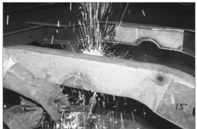
▲ After tracing the profile of the kit's curved section, each rail is notched. Installed notch plate and frame gusset are visible on far side.
