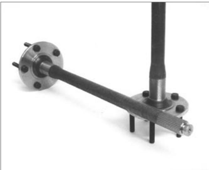
▲ Moser "C"-clip rear axles were built to exact length for the narrowed 12-bolt rearend. Moser Engineering (Portland, Indiana) also supplied studs and bearings.
