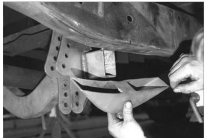
▲ The front 4-link brackets are welded to the trimmed crossmember, which then installs under the frame. Next, each "U"-bend gusset is welded to the crossmember and frame.
