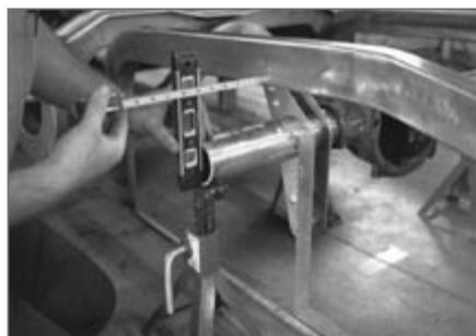
▲ With the new subframe in place, the narrowed rearend housing is positioned and centered in the frame, using tapes, squares, and the reference surface. Lines marked on the frame at the beginning of the project.
