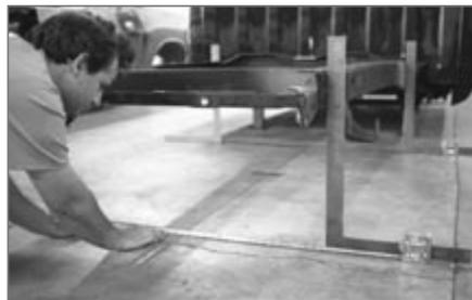
▲ A piece of string is one of the most important tools in this rebuilding procedure. With the frame stripped to the bone and the truck at the desired ride height, squares and tapes are used to find the center of the frame front and rear, and the string is taped to the floor on those marks.
