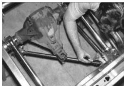
▲ With the link bars and the shocks in place, the installer checks for freedom of suspension travel by blocking up one end of the housing and applying all of his weight on the other end.
