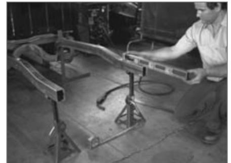
▲ Once both frame rails are tacked in place, the rear sections are checked to verify that they are level.
