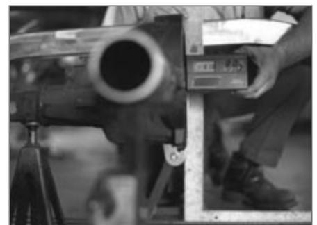
▲ The pinion angle is set at 1-to-2 degrees downhill by using a protractor set against the rear-cover mounting surface.
