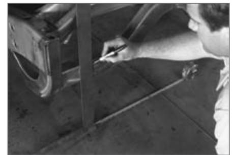
▲ Using the string line, tape and square once again, the position of the rear frame rail, as determined by tire size, is marked on the raised crossmember.
