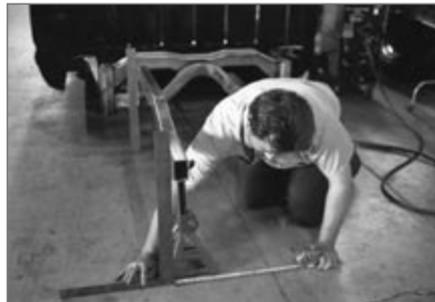
▲ With the front of the new frame rail tacked to the raised crossmember, the rear of the rail is positioned at the desired ride height and the correct distance from the string line.
