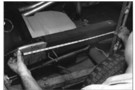
▲ After the bed is removed and the undercoating scraped off, the main reference line is marked 24 inches forward of the rear-axle-housing centerline.
