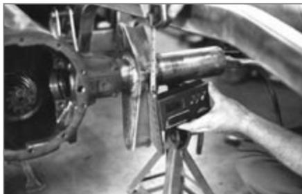
▲ After welding both the bracket to the axle tube and the included gusset plate to the back of the bracket, the lower shock mount is tacked onto the gusset. The height of the shock bracket itself is determined by the desired ride height, and it angles inward 10 degrees.
