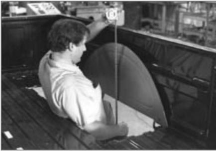
▲ The 20-gauge Chassisworks steel truck tubs are shipped preassembled (and in fairly large boxes!); here, a template is used to measure and scribe the cutting line on the inner bed wall.
