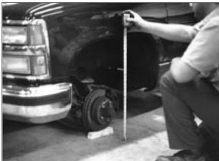
▲ The front end is blocked up at its new, substantially lower ride height, as measured at the top of the fender well, as the truck is prepared for this project.
