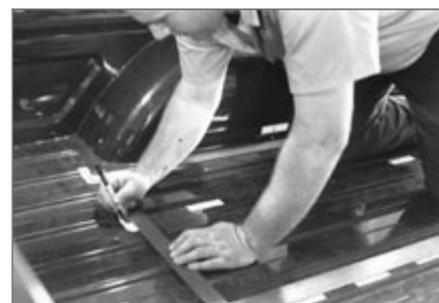
▲ Using strategically placed strips of white tape to aid in the effort, the bed is measured for the installation of the Chassisworks truck tubs. Before the bed was removed, a locating hole was drilled through the stock wheel well, above the axle centerline.
