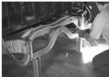
▲ The raised crossmember is cut to fit and welded in between the two drop loops. The high point of the loop is positioned directly above the driveshaft.
