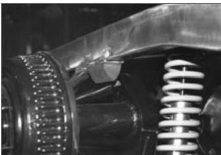
▲ The stock rear-axle snubbers are trimmed down to the bare essentials and welded to the bottom of the frame rails.
