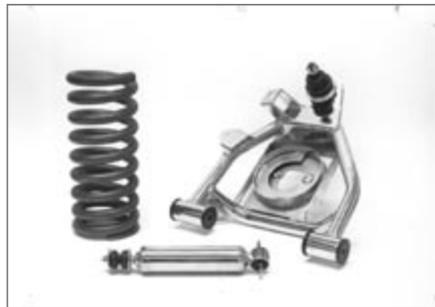
▲ This Chisholm 4-inch drop kit (two inches from the lower A-arm and two inches from the dual-rate spring) will be installed up front to keep the truck level once the rear is lowered.
