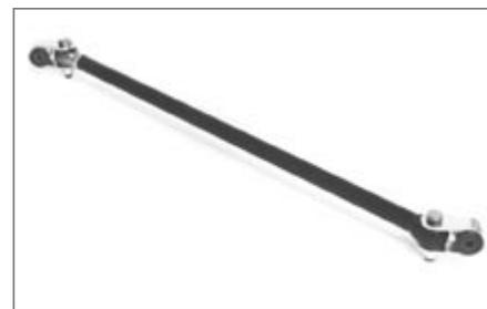
▲ Chassisworks has developed trick, urethane bushed double-clevis ends for the track locator. Allowing the locator to pivot in any direction without binding, these eliminate the problems associated with street use of race-bred track locaters or panhard bars.
