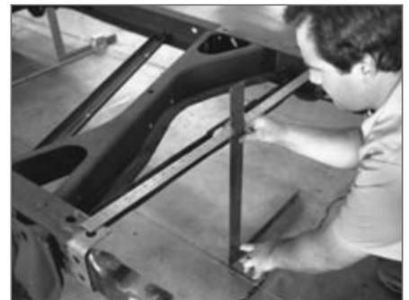
▲ A square is used to help find the distance from the string center line to the rear bed-mounting holes. A measurement is also taken from a reference point up front.
