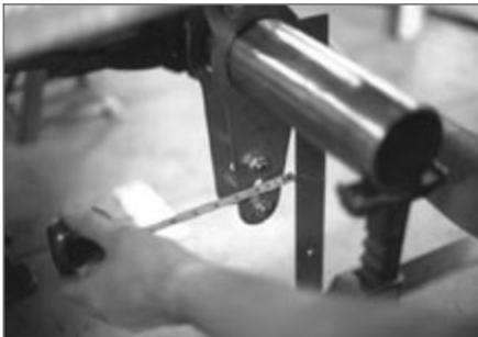
▲ The rear 4-link brackets are then assembled and tacked in place, using the steel sleeves from the urethane rod-end bushings as spacers. The location is determined according to the Installation instructions and assembly drawings, which take into account wheel and tire size and the amount of wheel backspacing; the middle mounting hole lines up directly beneath the axle-tube centerline to set the correct rotation.
