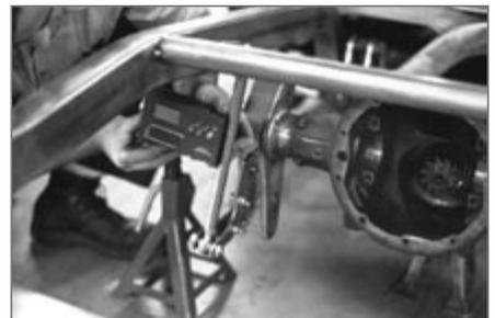
▲ The upper shock mounts and crossmember are positioned so the shock is dead-on vertical front-to-back, while leaning inboard 10 degrees. A shock simulator is used here to facilitate these alignments.
