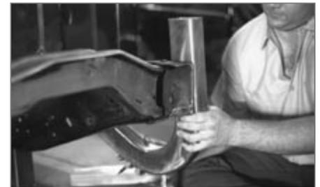
▲ With the frame torched off and ground smooth, this 120-degree drop loop is positioned the specified distance from the ground for the new ride height, and then marked for cutting. When installed, it will be on the inside of the frame rail.
