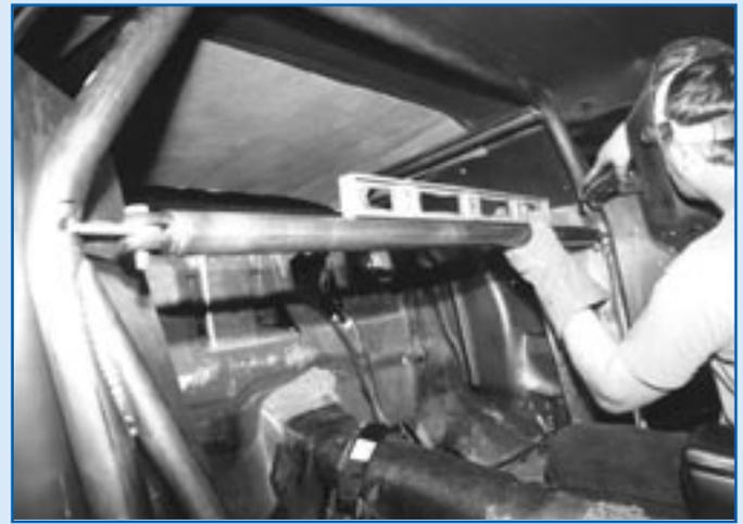
The mounts for the back brace are positioned at the widest point of the main hoop. One end of the tubing is fully welded to the clevis, while the other is left loose until the very end of the fitting-and-installation process.
