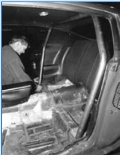
With the floor plates welded to the floor, it's time to fit the main hoop and contour the ends to fit the plates. The roll bar was leaned back slightly, to match the angle of the door opening; it should sit as high as possible in the car, while still allowing enough room to fully weld the rear struts to the hoop.
