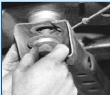
Installing the subframe connectors is the next step. This is what the box-tube subframe connectors look like when they arrive, complete with factory-welded mounting gussets and end caps.
