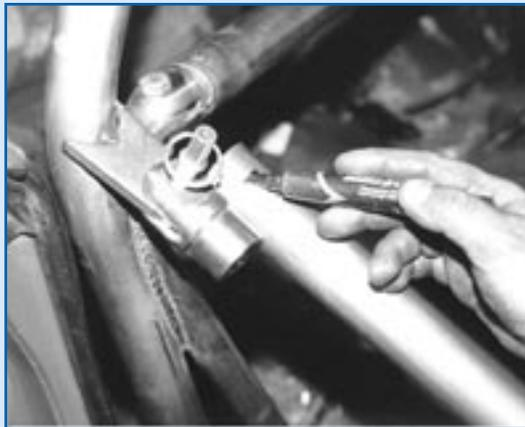
With the mounting tab now tacked to the hoop, the tubing is marked for its second cut.
