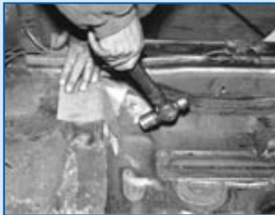
Floor-plate material for the roll bar is included in the kit. After being cut to size, the plate is then formed into shape. Also visible in the foreground is the top of the subframe connector, welded to the floor.
