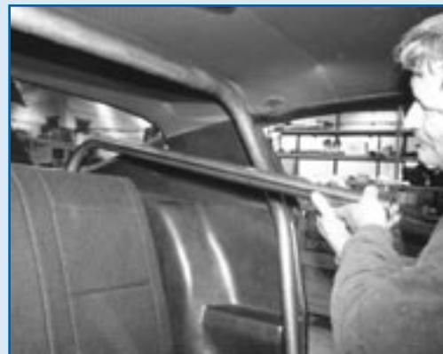
Fitting the bent rear struts is the next part of the installation process; the hidden end of the pre-bent tubing goes through a hole in the rear package tray and rests on a floor plate. Note: When marking any tubing for cutting to length, leave it a bit long and then "sneak up" on the proper fit with a series of short cuts.
