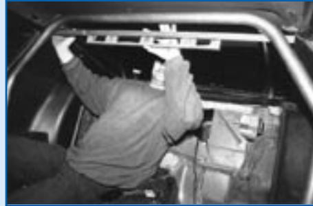
After both rear struts are fabricated and in place at the middle of the main hoop's bends, a straightedge and level are employed to make sure both sides match.
