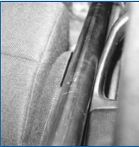
With the seat mocked up in place, another critical item to check before welding everything up is the clearance between the side bar and the arm rest. Failure to do so may result in some unnecessary hacking of the door panel.
