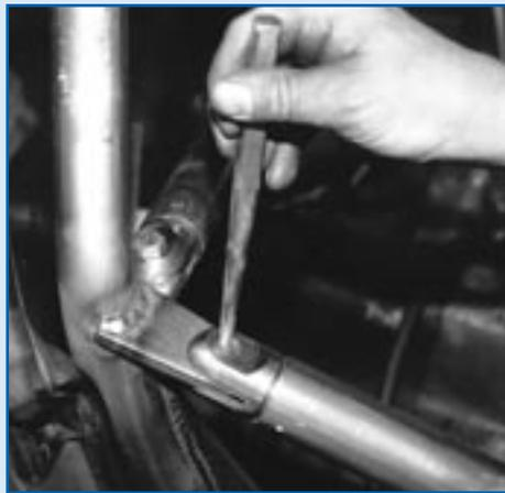
After welding the tab to the main hoop and cutting the side-bar tubing to length, the clevis is installed in the end of the tube and the holes aligned with the help of a punch.
