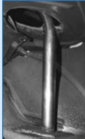
This view from the trunk shows the strut in place and fully welded to the mounting plate.
