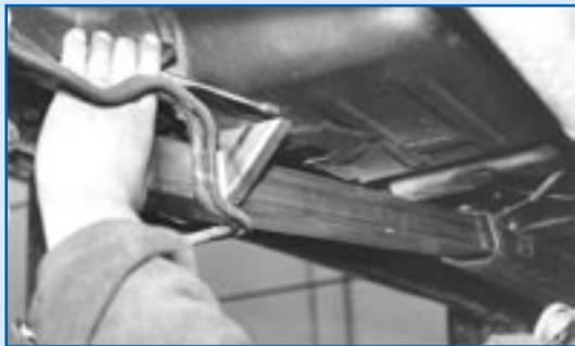
After bending the brake lines out of the way, the connector is ready for welding. The gussets on either side of the connector may have to be notched to follow the contour of the floor.
