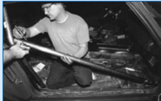
After determining the best angle for the side bar, the front assembly is tacked down; here, the rear mount is held in place and the tubing marked for cutting.
