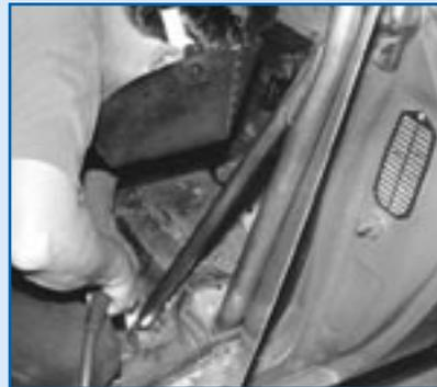
The hole in the floor must be large enough to allow the strut to be welded to the subframe connector itself.
