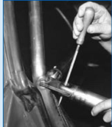
We recommend using a round file or die grinder, rather than a larger drill bit, to "egg-shape" the hole in the mounting tab to achieve proper quick-pin clearance if the alignment changes due to the welding procedure.
