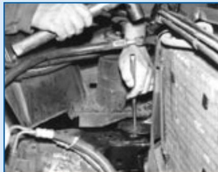
After removing the bolt that holds the body bushing in place, the rubber OEM piece is pounded out.
