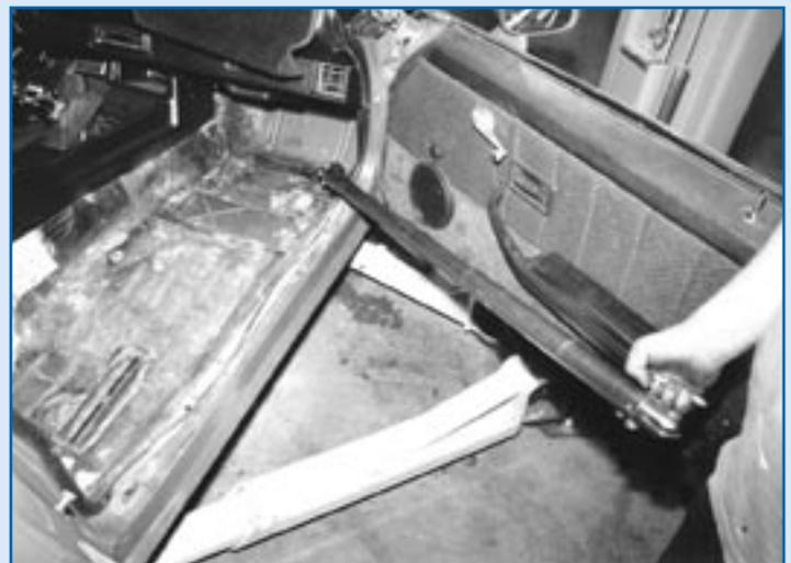
Before doing any final welding, the side bar is checked for proper operation and orientation.
