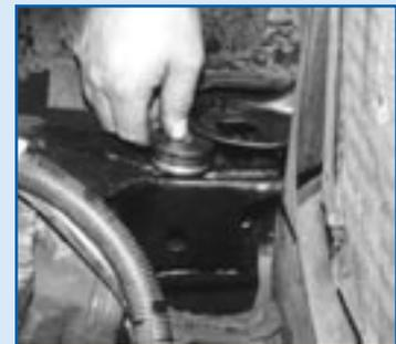
The billet bushing then slides into place and is bolted down. Caution: Don't remove all the bushings on each side at the same time, or the body and frame will have to be realigned.
