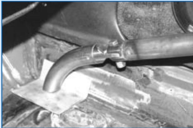
Again, the floor plate is cut and contoured; the lower end of the bar itself is fully welded and bolted to the bracket, while the bracket itself remains loose in the tubing until the fit is finalized.
