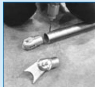
When fabricating the bars for both the removable back brace and the swing-out/removable side bars, a hole is drilled through the end of the tubing for a rosette weld before inserting the clevis.
