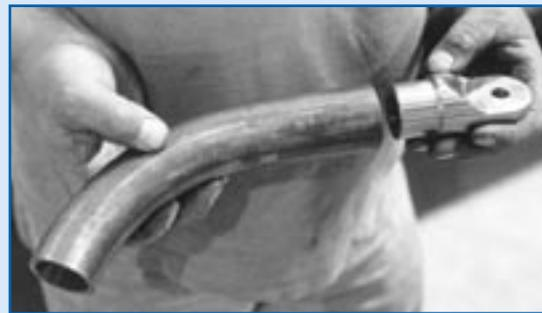
This combination of tubing and bracket is used to provide the front mounting/pivot point for the side bars.
