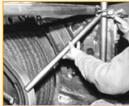
The next order of business is to fabricate the struts from the main hoop back to the new subframe rails. With the lower end of the tubing roughly in place on the top of the subframe bend, the top of the tube is marked with the angle required to have it fit fairly snugly under the back-brace mount.
