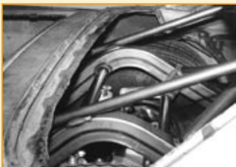
After welding the struts front and back, they were also raised part of the subframe rails since they line up so closely in this early Nova kit.
