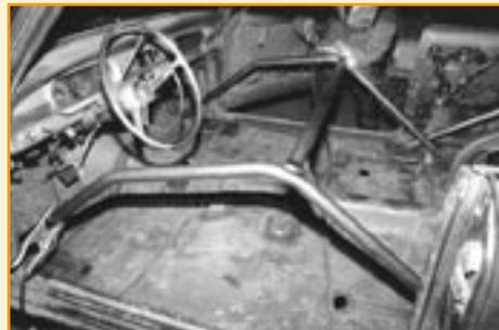
The cage side is cut to fit and positioned; the form-following shape of the tubing in the early Nova kit can be seen in relation to the windshield post.
