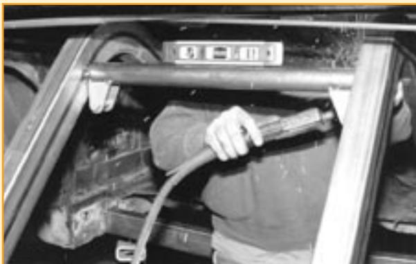
The upper shock mount is fabricated as per the instructions, positioned as referenced from the dropped crossmember, and tacked to the frame rails. (The use of a level that attaches to the tubing magnetically is recommended, but you must make sure that there are no metal shavings between the level and the tubing.)
