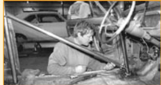
Because this Nova will be seeing considerable street time, swing-out side bars are being installed along with the removable back brace. Here, the swing-out clevis is welded to the lower end of the tube, bolted to the mounting tab, and, with the top end of the tube resting roughly in place, the tab is about to be tacked to the cage-side tubing.
