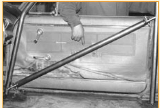
After cutting the side bar to length and installing the upper clevis, but before everything was welded up, the door was closed to make sure that the side bar didn't interfere with the operation of the door and window handles. As shown here, the handles are fine; however, the stock arm rests are history.
