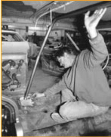
Both cage sides are in place, and the windshield brace is marked for cutting.
