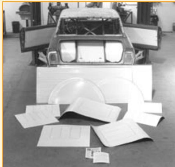
All of the pieces used in a typical tin-installation project are laid out here, including the detailed instruction sheets. Not shown is the steel driveshaft tunnel.
