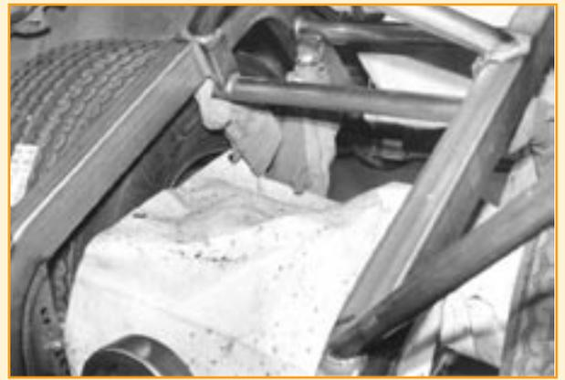
Our exclusive antiroll bar was also installed in the Nova. This is the completed assembly after it was fabricated; the box-tube mounting brackets fit inside of, and are welded to, the new subframe rails, while the width of the arms exactly matches the outer width of the frame. Pieces of thin steel plate are included for capping off the cut-to-size mounting brackets.
