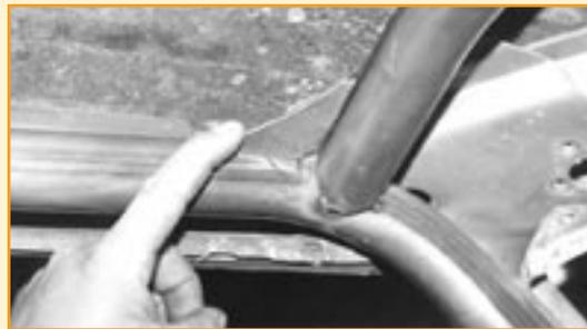
After tacking both sides of the main hoop in place, it is checked to make sure it is level before moving on to the cage sides.
