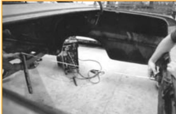
Next, the distance from the trailing edge of the crossmember to the inside of the rear of the car, in the trunk area, is determined. The rails will rest on the lip left behind when the trunk was cut out.
