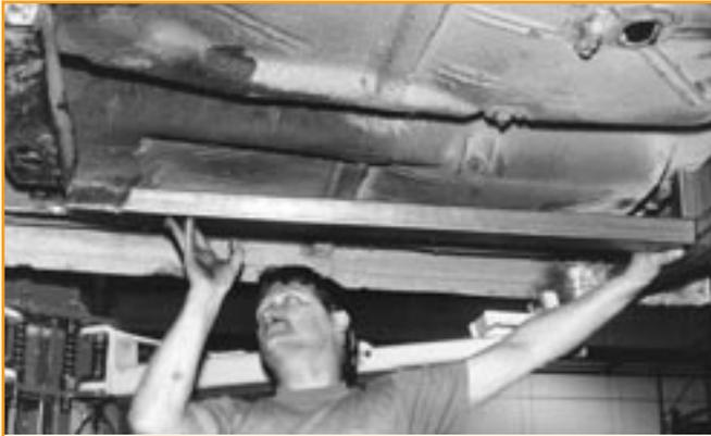
The floor of the Nova needed only a few taps with a mallet to make room for the connectors, while some other cars will require the floor to be notched. Note that the connector fits under the “overhang” of the frame rail, and is lined up with its inside edge.
