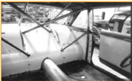
The installation of interior tin is covered elsewhere in this catalog, but this is what the interior of the Nova looked like when it was fully skinned. All panels are aluminum, and still covered with the protective plastic; the driveshaft tunnel is steel and welded to the floor. Cleco clips are being used to hold the panels in place, prior to the actual riveting.
