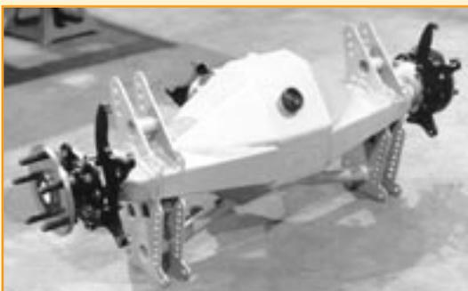
Here is the Chassisworks FAB9 rearend housing, complete with 4-link brackets and back braces, that was used in the Nova. Installing the center section, axles, and brake-kit brackets before mounting the housing is recommended.
