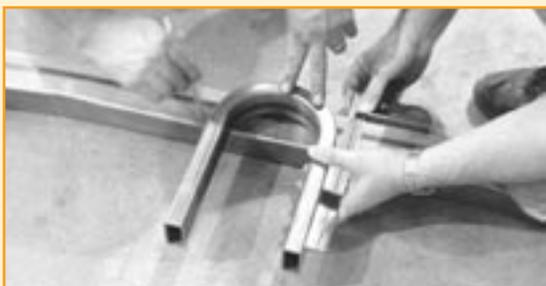
The driveshaft centerline is marked on the crossmember (along with identifying the passenger and/or driver's side of the crossmember to assure its orientation); the bottom half of the driveshaft loop is centered on the crossmember at this point, with the bottom of the loop lined up just above the bottom of the crossmember, and the 3x2-inch tubing is marked for notching. The use of a square will ensure proper alignment.
