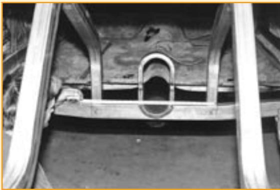
The frame rails are placed with their outside edges on the lines on both the crossmember and the inside of the trunk lip, tacked in place, and again measured to verify the proper width. Measuring across the tops of the frame rails should also be done to verify they are plumb and straight.
