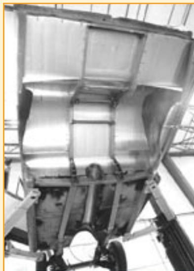
With the Nova high on the lift of our in-house chassis shop, this snail's-eye view shows how the tin installation, the dropped crossmember, and the subframe connectors all tie in together to provide a sanitary package.
