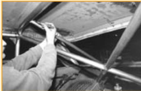
The rear of the strut will be installed on top of the extreme rear of the subframe rail, flush with the outer edge. Once the leading end of the strut is in place, a straightedge is clamped to the top of the rail at the midway point to help line it up.
