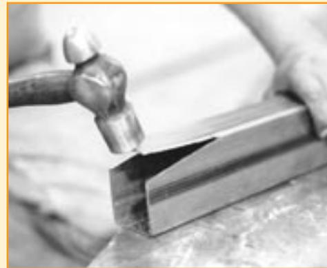
Since the front-frame stub is narrower than the box tubing, the front of the connector tube was notched to provide the proper contour; the "flaps" will be hammered down and welded, with the welds then ground smooth.
