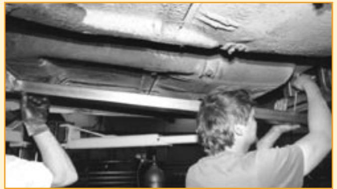
After the frame stub is removed, the 3x2-inch box tube to be used for the connector is held up in place and the trailing end marked for cutting. As always, a snug fit aids in the installation process.
