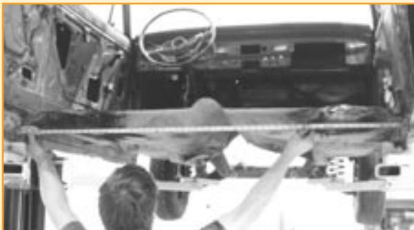
The crossmember will reside between the rocker panels of the unibody Nova, along the lower edge. When measuring for the proper width of the crossmember, be sure to note the location of the driveshaft centerline, which is rarely in the exact center of the car.
