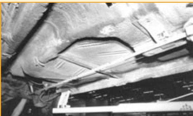
Reference points are also critical under the car for fabricating the new subframe; in this instance, the front of the transmission crossmember-mount is the fixed point choice used for measuring back to the front of the axle housing.
