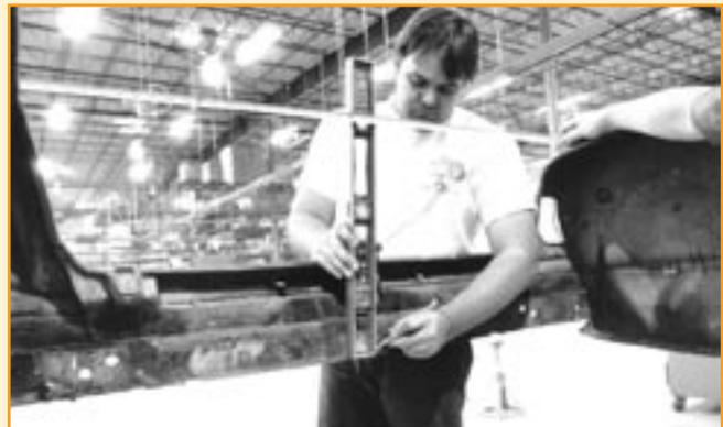
Assuming the body is unwrinkled and the rear quarter panels are straight, a tape is used to measure across the back of the car to find the exact center of the rear area. It can't be assumed that the trunk-latch mechanism is in the middle of the car.
