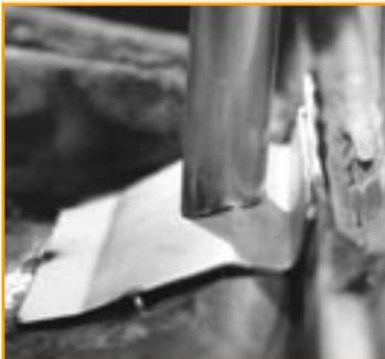
With the windshield brace positioned and tacked to the cage side, these corner gussets, included in the kit, are added to the structure.
