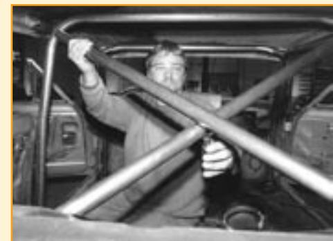
The next chore is the fabrication of the X-braces. The area at the top of the antiroll-bar mount was designated as the spot to mount the rear of the brace, while the forward end will attach right in the middle of the main-hoop bend, in line with the cage-side tubing. After the first, continuous-length brace was cut, formed and tacked to the car, the second piece of X-brace tubing is marked to start its fitting procedure.
