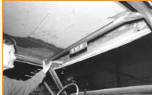
This is how the end of the main-hoop tubing was notched to fit the plate's contour. The weld will fill in any gap (within reason, of course) that exists between the pieces.
