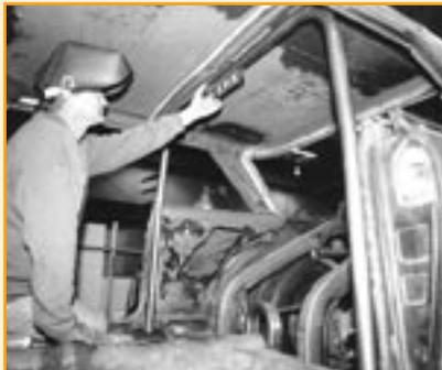
Here's the aforementioned method for welding the top of the windshield-brace joint. The tack welds holding the cage-side/windshield-brace assembly to the floor and to the main hoop are broken, the assembly is set down on the floor, and the welding can be easily done. (The tacks holding the main hoop to the floor will probably also have to come loose for this process.)
