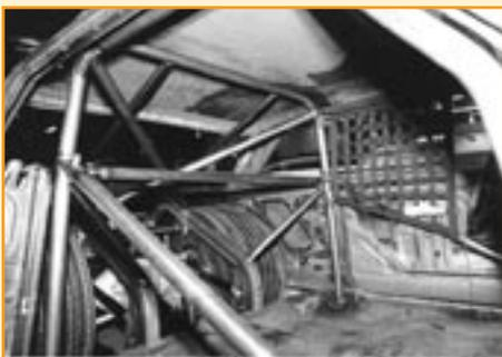
This view into the Nova's passenger compartment shows all the tubing of the 10-point roll-cage kit in place at the completion of the project.
