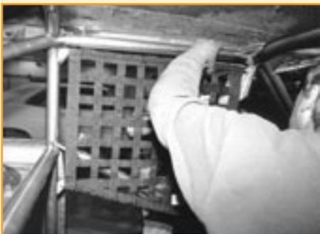
The upper, rear mounting tab for the window net was welded right next to the gusset at the intersection of the main hoop and the cage side; the lower, rear tab was mounted to the main hoop, as shown. Here, the proper location for the clevis for the quick-release pin is determined.
