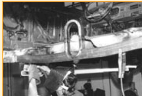
The completed crossmember is worked into position, with the bottom of the crossmember's ends flush with the bottom of the rocker panels, and tacked into place. If the crossmember has been cut to achieve a snug fit, the positioning and alignment of the crossmember is much easier.
