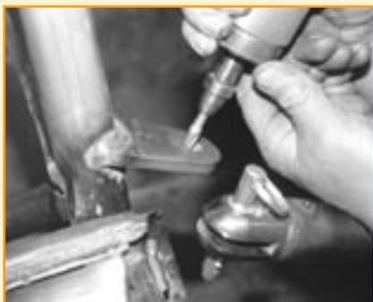
With the welding completed, the front seats are mocked up in place. The removable back brace will be the mounting location for the top straps of the intended 5-point safety harness.
