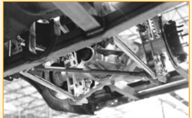
...while this shot from under the car shows the track locator in place, along with how the subframe connectors meet the crossmember.
