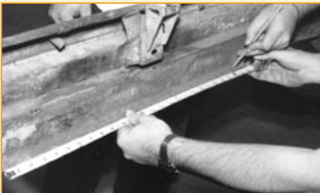
Once the midpoint of the car is established, the proper distance is measured out in both directions from this point, to mark the location of the frame rails (in this application, they will be 24 inches apart, as measured from the outside of the rails).
