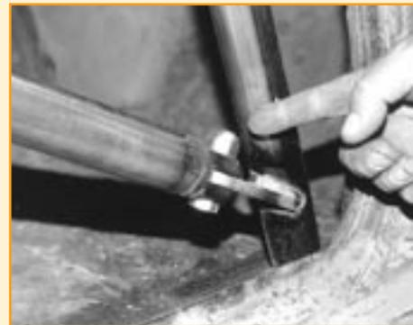
The nut has to be located at the top in this case, or the bar will never be able to be removed. The angle and position of the lower mount must also allow the intended operation of the swing-out arm.
