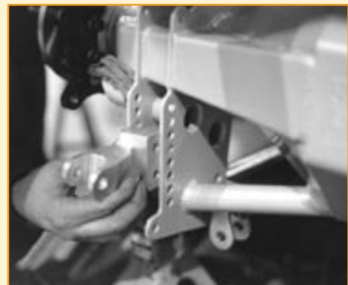
The billet, CNC-machined lower shock mounts are installed on the housing, again starting off by using the middle set of bracket holes.
