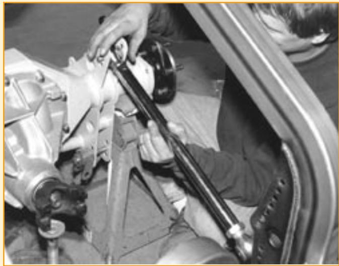
With the housing resting roughly in place and the pinion angle established with the help of a protractor and screw-type jackstand, it's time to install the link bars. The middle set of holes on each bracket is used for the initial set up, and all the bars are positioned with their threaded rod ends in the forward location, to facilitate later fine-tuning of the suspension.
