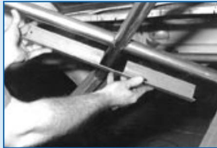
Next, a strut connects the main hoop to the frame above the 4-link bars, forming an X-brace. Chassisworks installers use this notched section of angle iron to align and hold the three sections during welding.
