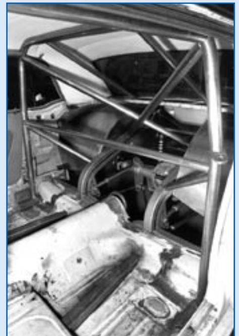
In this trial-fitting, both tubs are temporarily attached to the frame with Cleco clips.
