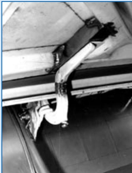
Closeup reveals reworked hinge and fabricated box mount, welded to the deck lid. The original spring latch was shortened and attached to the cage strut.
