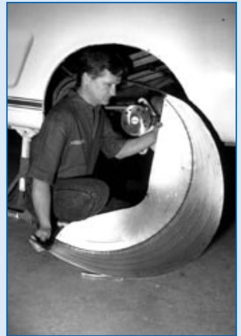
After determining the largest tire diameter (29 inches) that would fit inside the stock wheel openings, tinsmith Jimmy Berg selected a pair of 24x40-inch Chassisworks aluminum tubs.
