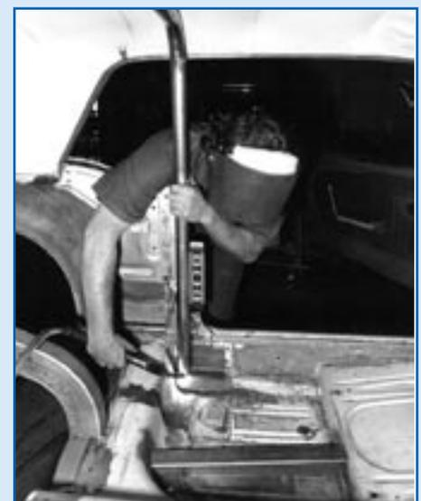
After tack-welding the floor plates, Garceau uses a magnetic level while tacking the main hoop.
