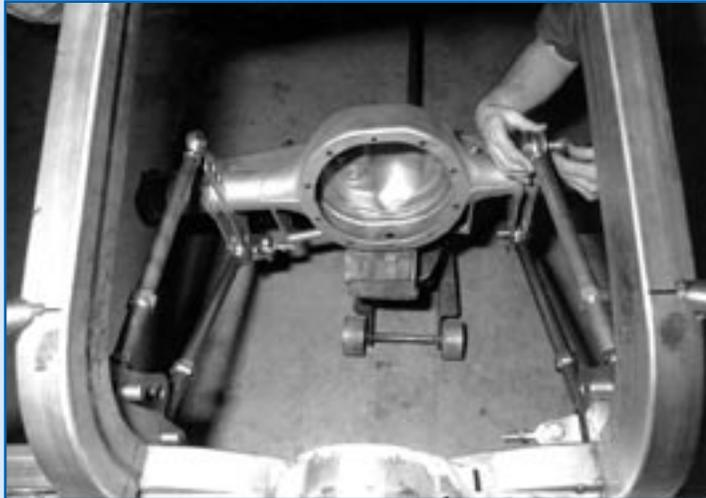
After bolting both coil-spring assemblies to their lower brackets, Joel raises the entire rearend to align the upper shock mounts with the crossmember.
