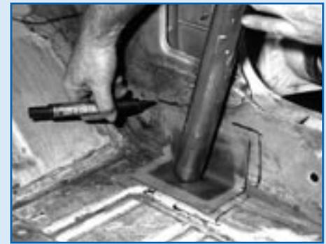
Roll-cage construction begins by bending four 1/8-inch floor plates to the contour of the floor. These will anchor the cage sides and main hoop. Once the prebent tubing is cut to length, an area slightly larger than each plate is marked off, as shown.
