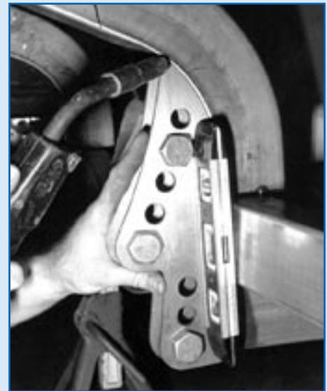
Suspension stage begins by tacking in both sets of forward 4-link brackets, even with the outside of the frame rails.
