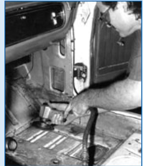
To ensure the best possible weld, each outlined area is ground to remove any paint, body filler or debris.
