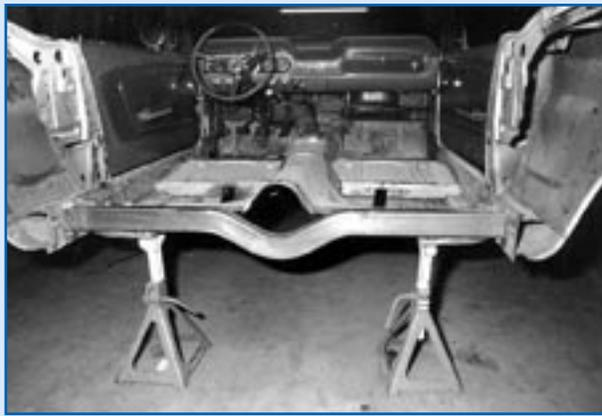
Next, installer Joel Garceau trims and installs both subframe connectors through the corresponding slots in the floor.
