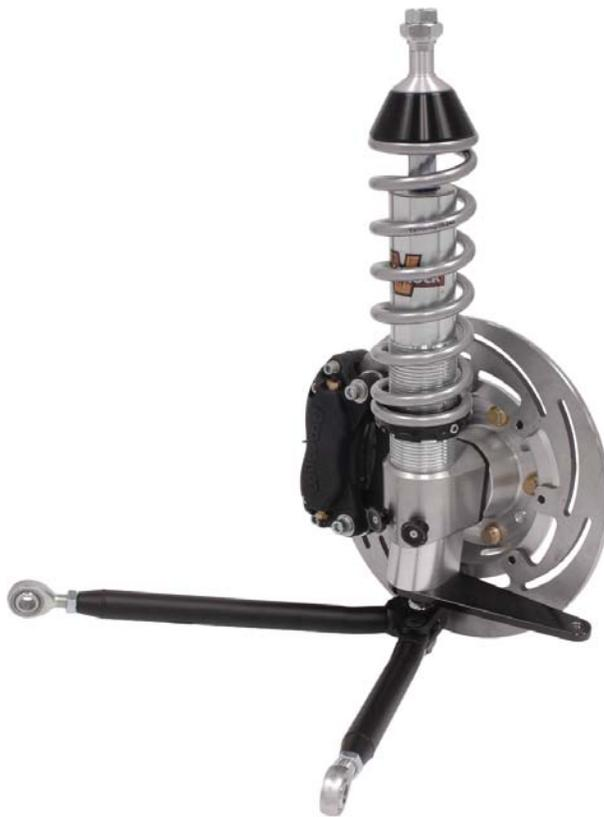
**DESCRIPTION:** DRAG QUICKSET 2, 6" TRAVEL, STEM STRUT SPINDLE SUSPENSION SYSTEM, INCLUDES QUICKSET 2 INTEGRAL SPINDLE, 3/4 x 5/8-18 STEM MOUNT, 6" TRAVEL STRUT, CONTROL ARM, BRAKE KIT, AND SPRINGS
