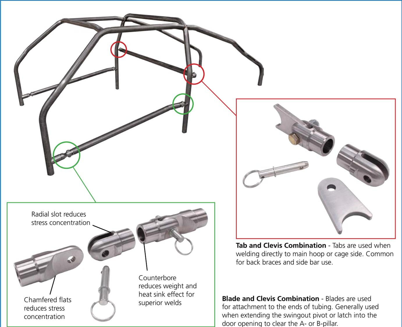
**Tab and Clevis Combination** - Tabs are used when welding directly to main hoop or cage side. Common for back braces and side bar use.
