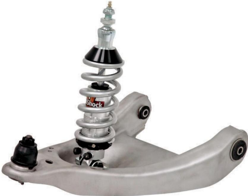
This is a pretty traditional shock mounting arrangement, but VariShock has dozens of mounting arrangements that allow the shocks and coilovers to bolt into just about any American car made since the late '50s.
