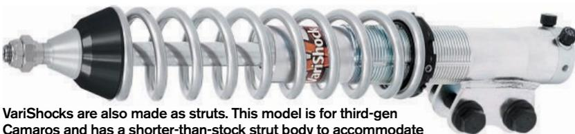
VariShocks are also made as struts. This model is for third-gen Camaros and has a shorter-than-stock strut body to accommodate lowered cars.
