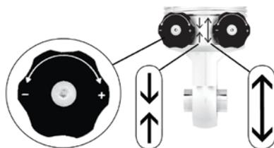
A double-adjustable shock, on the other hand, comes with two knobs and allows rebound and compression damping to be adjusted independently of each other.
