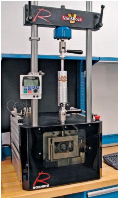
Chassisworks makes extensive use of its state-of-the-art shock dyno for research and development. Every VariShock is also tested and calibrated to strict performance guidelines before it's shipped to the customer, ensuring that each shock performs as it should.
