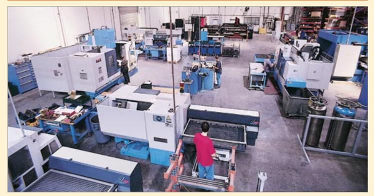
Numerous Chassisworks parts are produced entirely on our Mazak flexible manufacturing cells. These incredible machines represent a quantum leap in technology from the old-style CNC lathes used by many manufacturers. Each machine is a combination of two lathes and two mills, with automatic material loading
