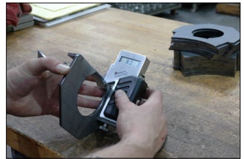
▲ Each part is QA checked using measurement devices or a physical-fit gauge. Any variances will be corrected before moving on to welding.
