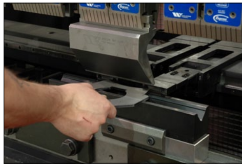
▲ The automated back stops move to various positions and allow the same bend die to be used on parts with multiple angle bends or varying degrees.
