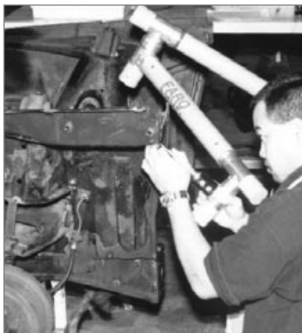
▲ The operator then runs the probe over the surface of the object being scanned; every time a button on the arm is pushed, the coordinates are recorded. Here, the locations of the bolt holes for mounting a Nova front end to the firewall are plotted.
