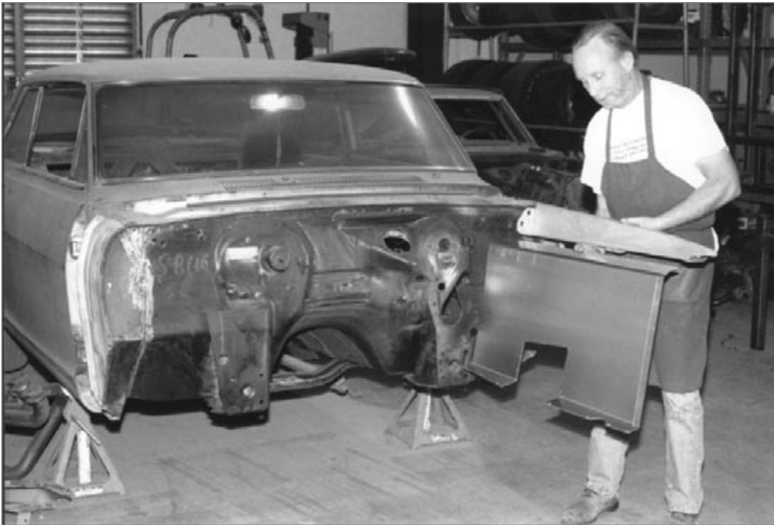
▲ The fender/hinge mount is then checked against the test-mule Nova used for acquiring all of the dimensions for this project, along with one of the new aluminum Inner fender panels.
