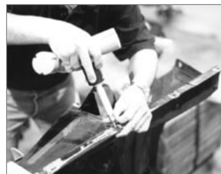
▲ Here, the all-important mounting bosses for the outer fender panels are located, along with the curve of the surface itself. This information was critical in manufacturing the upper fender/hood hinge mount.
