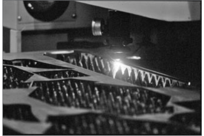
▲ This laser cutting machine is amazing to watch. The sparks fly as the initial hole is burned in the steel plate, after which a gentle glow is all that is seen as the laser cuts the steel with an incredible precision.
