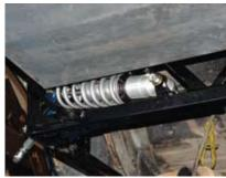
The VariShock coilover is in place. As previously noted, the outer body of the shock is threaded, and the dark collar at the bottom of the spring can be turned to raise or lower the spring as well as adjust the ride height accordingly.
