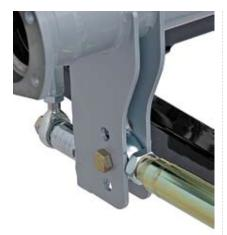
This factory photo shows how the other end of the trailing arm attaches to the axle bracket using spherical joints, which offer zero deflection. The length of the trailing arm is adjustable at this juncture, and the adjustment is locked into place with the large jamb nut.
