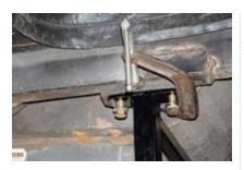
Install the shockabsorber rocker arms. Here, we view the job from outside the wheelhouse looking in. The top of the rocker arm attaches to the shockabsorber end, and the spherical joint connects with the axlehousing. All of the fasteners will be tightened to 50 ft-lb. ▶
