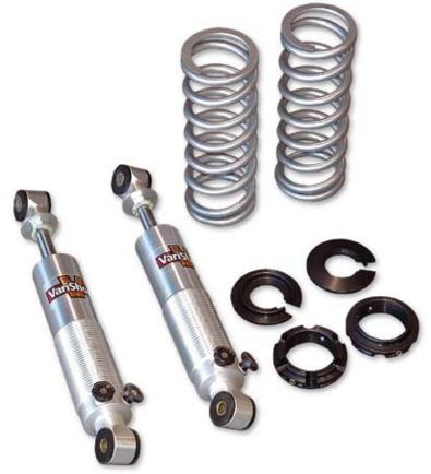
Here's a close-up of the coilover shocks. Besides allowing the ride height to be dialed in exactly via the threaded adjustment collars, they're also externally adjustable for both bump and rebound in a range covered by 16 increments.
