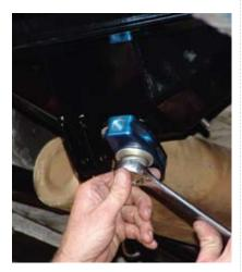
The pivot arm for the Watt's linkage is mounted to a threaded boss welded onto the bottom of the FAB9 housing or to your supplied housing.
