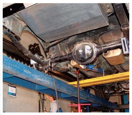
The TCP kit replaces the entire rear suspension, so it's necessary to remove all of the old hardware prior to installation. Remove any portions of the exhaust system that may interfere, although mufflers can remain in place if in the stock location. Definitely unbolt or cut any exhaust tubing that's routed over the rear axlehousing.
