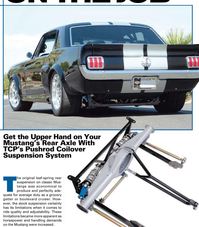
When performance-oriented people install larger wheels and tires out back, it becomes clear that the leaf springs are a limiting factor when it comes to selecting a tire and offset for any kind of high-performance application, be it road racing, drag racing, or just spirited driving. The original leaf-spring suspension also allows serious axle windup, and it does a poor job of locating the axle precisely in relation to the chassis during turns.
