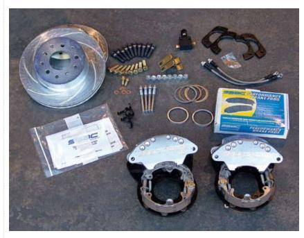
During the course of the conversion, we'll also install these rear disc brakes from Stainless Steel Brakes Corp. Included along with the calipers are slotted rotors, parking-brake assemblies, and braided steel brake lines.
