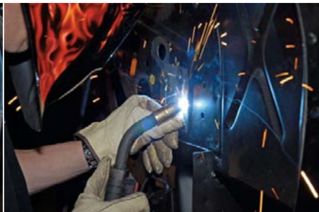
Installer Martin first creates a weld-in "blank" which is initially tack-welded in place. After checking the fit it gets hammer welded in position.
