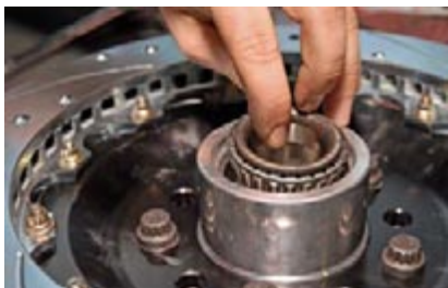
Next, comes the installation of the front bearing, again using an ample supply of high quality wheel bearing grease.
