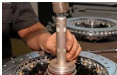
The bearing races are pressed into the billet hub at the factory. After packing the inner wheel bearing with a high-quality wheel bearing grease, our installers use a hammer and a seal installer to drive the seal into the hub.
