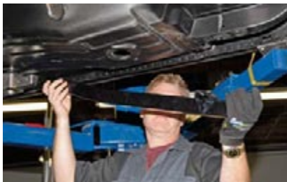
Woods trial fits the Alston sub frame connectors (p/n 5601-20) up to the underside of our Dynacorn Reproduction Bodies '67 Camaro uni-body.
