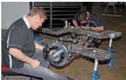
Next, Dan installs the passenger side Wilwood disc brake caliper using the 3/8-16 x 1-3/8-inch socket head Allen's, lock washers and flat washers provided in the kit.
