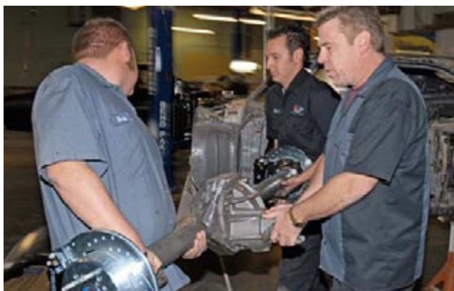
On the opposite end our crew installs the OE reproduction spring bucket for the Camaro rear leaf springs to "sit" in using the OE bolts provided.
