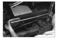
▲ After the bed Is removed and the undercoating scraped off, the main reference line is marked 24 inches forward of the rear-axlehousing centerline.
