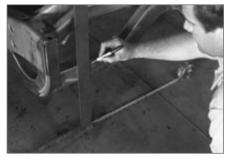
▲ Using the string line, tape and square once again, the position of the rear frame rail, as determined by tire size, is marked on the raised crossmember.
