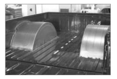
▲ The available cargo space in the pickup bed takes a beating after the tubs are installed, but the result is truly an impressive sight. The tack-welds can be seen on the tub on the right, while the other has already been completely welded.
