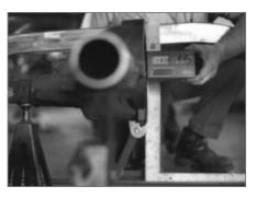
▲ The pinion angle is set at 1-to-2 degrees downhill by using a protractor set against the rear-cover mounting surface.
