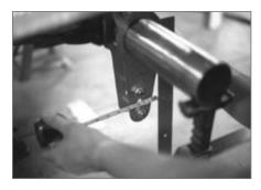
▲ The rear 4-link brackets are then assembled and tacked in place, using the steel sleeves from the urethane rod-end bushings as spacers. The location is determined according to the Installation instructions and assembly drawings, which take into account wheel and tire size and the amount of wheel backspacing; the middle mounting hole lines up directly beneath the axle-tube centerline to set the correct rotation.
