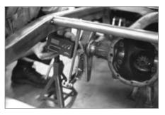
▲ The upper shock mounts and crossmember are positioned so the shock is dead-on vertical front-to-back, while leaning inboard 10 degrees. A shock simulator is used here to facilitate these alignments.
