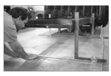
▲ A piece of string is one o the most important tools in this rebuilding procedure. With the frame stripped to the bone and the truck at the desired ride height, squares and tapes are used to find the center of the frame front and rear, and the string is taped to the floor on those marks.
