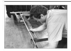
▲ After installing the rear crossmember, the rear bed-mounting brackets are located and attached. These brackets, as well as the additional braces and gussets, are fabricated from the pieces left over when the main frame tubing is cut to size.
