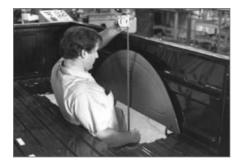
▲ The 20-gauge Chassisworks steel truck tubs are shipped preassembled (and in fairly large boxes!); here, a template is used to measure and scribe the cutting line on the inner bed
