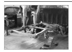
▲ With the link bars installed and adjusted, the welded end of the unique Chassisworks Pro Street track locater is marked for cutting to the proper length.
