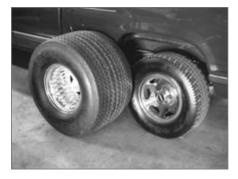
▲ The stock wheels and tires are dwarfed by the MIT Sportsman 33x21.5-15 tires, mounted on Center Line 15x15 Convo Pro wheels, that will replace them on the rear.
