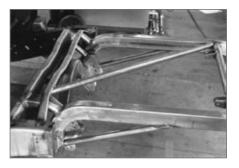
▲ All of the extra bracing required to stiffen everything up can be seen here. Tubing for the diagonal and the lower braces is included in the rear-sub frame kit, while the shorter braces are fabricated from cut-off pieces of the sub frame components.
