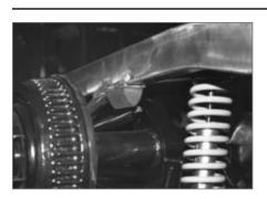
▲ The stock rear-axle snubbers are trimmed down to the bare essentials and welded to the bottom of the frame rails.
