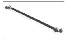
▲ Chassisworks has developed trick, urethane bushed double-clevis ends for the track locater. Allowing the locater to pivot in any direction without binding, these eliminate the problems associated with street use of race-bred track locaters or panhard bars.
