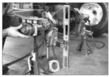
▲ The narrowed housing is then removed from the frame to have the axle flanges welded back on. Here, a couple of levels and the Chassisworks rearend-narrowing fixture are used to align the flanges.
