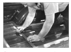
▲ Using strategically placed strips of white tape to aid in the effort, the bed is measured for the installation of the Chassisworks truck tubs. Before the bed was removed, a locating hole was drilled through the stock wheel well, above the axle centerline.
