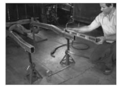
▲ Once both frame rails are tacked in place, the rear sections are checked to verify that they are level.
