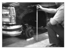
▲ The front end is blocked up at its new, substantially lower ride height, as measured at the top of the fender well, as the truck is prepared for this project.
