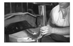
▲ With the frame torched off and ground smooth, this 120-degree drop loop is positioned the specified distance from the ground for the new ride height, and then marked for cutting. When installed, it will be on the inside of the frame rail.
