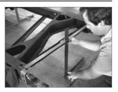
▲ A square is used to help find the distance from the string center line to the rear bedmounting holes. A measurement is also taken from a reference point up front.
