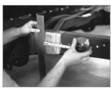
▲ This line, three inches to the rear of the 24inchreference point, Is where the stock frame rails will be cut off
