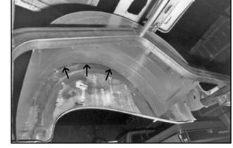
20 Nine Cleco clips temporarily attach the wheel tub. Ultimately, each will be replaced with a blind rivet, and a bead of silicone will seal the tub's rounded edge to the quarter panel.
