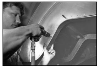
18 Each fully trimmed tub can be temporarily clamped or clipped to the frame while mounting holes are drilled 1" up from the frame, 2" apart for mounting rivets. (Note the Cleco pin attaching this tub at the frame's bend.)
