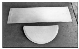
Here's one aluminum wheel tub as it comes out of wood-reinforced Chassisworks box. Thin plastic material protects both outside surfaces during trimming and installation.
