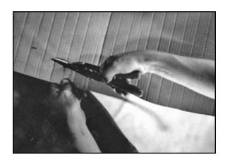
9 Cutting along the dotted line, Berg trims excess material from the top section.
