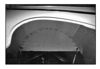
1 1 The secret to a clean, accurate installation is the included contour tool. The felt tip of a marking pen protrudes through the hole selected and enables a perfect line transfer.
