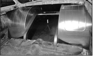
Here's a hot rodder's version of a "hot tub in the back." Together with a universal Chassisworks subframe, the new tubs nearly doubled this vehicle's original tire capacity.
