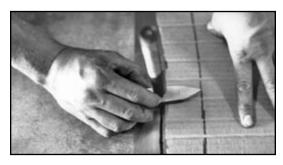
15 Next, the cardboard assembly is removed from the car and slipped inside the wheel tub. Reversing direction of the contour tool (but using the same hole as before), Berg transfers the body contour from the cardboard unto the metal top section, as shown. Consequently, the black line on the left becomes the actual cut line for the metal tub.
