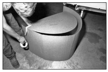
**7** Now the two cardboard sections are joined together with strips of masking tape.
