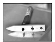
12 On each side of the body, Berg drags the contour tool along the inner quarter panel. As the point of the tool follows the body contour, the marker draws a corresponding black line onto the cardboard top section.
