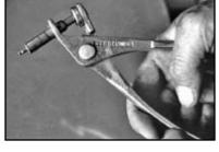
19 No installer should be without this inexpensive tool (available from Chassisworks). Reusable Cleco clips hold tin securely in place prior to and during the actual riveting.
