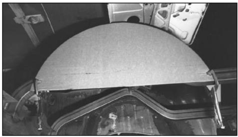
2 The cardboard shipping carton is used to make templates for each side of the vehicle. This section was made by tracing the end piece of the actual wheel tub onto the carton. The carton was then cut to exact size, and clamped against the Chassisworks subframe, as shown.
