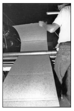
A straight, 24-inch-wide piece of cardboard will simulate each wheel tub's rounded top section. This pass through the Chassiswork metal roller made the cardboard easier to bend into an arc.
