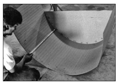
Directly opposite each measurement on the end piece, the corresponding distance is marked on the top section. These marks will form a dotted "cut" line.
