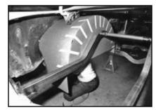
10 The assembled cardboard tub is clamped in place for final measuring and trimming.
