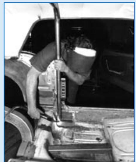
After tack-welding the floor plates, Garceau uses a magnetic level while tacking the main hoop.
