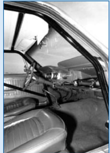
Black cage tubing complements the original red dashboard, door panels, seats and carpet. Optional, swing-out side bars are highly recommended for street applications. Notice how the cage sections do not interfere with the factory armrests, window cranks, door handles, sun visors or glove box.
