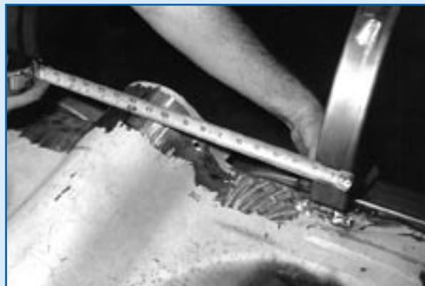
Cage sides are carefully positioned to clear the stock sun visors and glove-compartment door.
