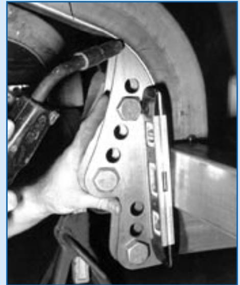
Suspension stage begins by tacking in both sets of forward 4-link brackets, even with the outside of the frame rails.
