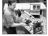
The FaroArm laser scanner is just one of the computerized measurement devices in Chassisworks' high-tech tool bin. With point and shoot ease. Chassisworks' laser scanner picks up fine details, such as casting imperfections, threads, and even tooling marks.
