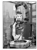
Robotic-spray arc welders consistently churn out error-free drag race products with strong and reliable welds.
