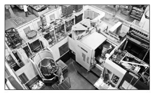
Chassisworks' manufacturing facility houses the latest in automated machining centers. This example features an automated two-tier fixture loading system and holds 160 different tools.
