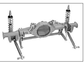
Engineered for stock-suspension drag racing classes, Chassisworks' FAB9 housings provide an easy conversion to the Ford 9-inch rear end and feature multiple mounting positions for instant-center and ride-height adjustment.
