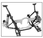
Chassisworks' 1962-67 Chevy II strut clip complete assembly lightly tips the scales at 124 pounds, including rack-andpinion, billet struts, and brakes.
