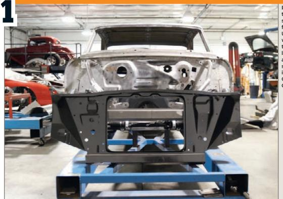
Pictured here is the new radiator support as received from Ground Up. Unfortunately, we must remove the support's lower core section according to the subframe installation instructions from Chris Alston's Chassisworks.
