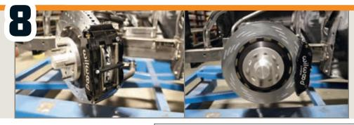
With the caliper mounted, it's a snap to install the brake pads. Bobby simply removed the nut, bolt, and spacer—which retains the pads—and slid them into place, then reversed the procedure. The rotor then spun freely, indicating that proper alignment had been achieved. Once Getaway is completed, we'll perform a series of tests to check the performance of these babies.
