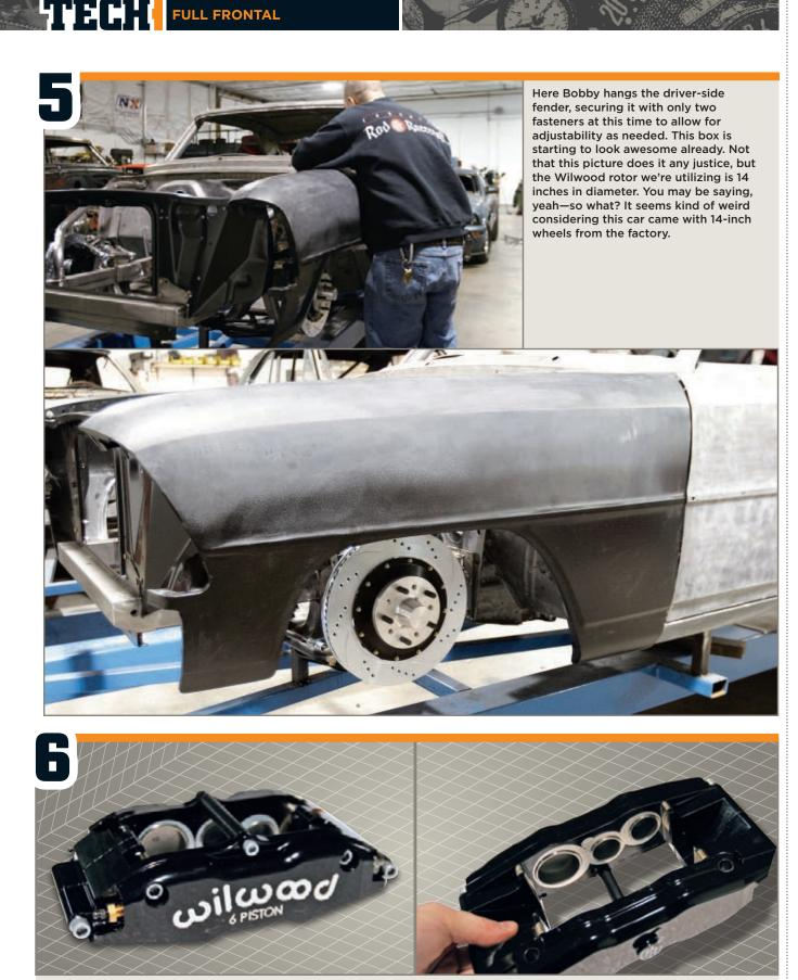
Speaking of the massive 14-inch stoppers, here's a peek at the Superlite SL6R Wilwood six-piston (under 5 pounds) caliper being used up front. This narrow unit features an increased bridge radius to allow for proper pad alignment and bridge clearance when using 13- to 14-inch rotors. Radial mounting makes for a cleaner installation and provides two planes of adjustment for ultimate alignment possibilities.
