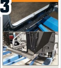
With the core removed, the support fit into the frame perfectly (as indicated). No further modifications were necessary to seat the unit. Bobby installed the three mounting bolts on each side of the frame through the integrated flanges.
