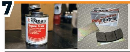
Before mounting the caliper, Bobby applied Bostik Never-Seez to the fasteners to ensure headache-free removal when needed. Once the caliper was mounted, we installed the Wilwood PolyMatrix disc brake pads. These particular units contain Wilwood's "Q" compound, which is ideal for disc brake conversions on street rods and musclecars. These pads offer improved friction over OE replacements as well as low noise and dust levels.
