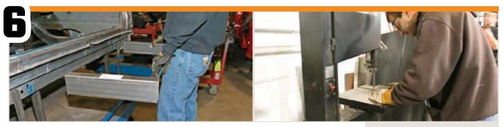
Here Bobby displays the additional length of frame that was removed. Since this piece contained the crossbar in the rear, it's advisable to tack in a new cross-piece further toward the front to keep the frame true during the installation. We caught Krawiec playing with something on the bandsaw. What the heck are you doing, Krawiec?
