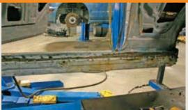
Shown here is our new Flintstone mobile (minus the stone wheels). Once the floor is cut around the edges, it's necessary to employ a drill bit—or better yet, a spot-weld cutter—to properly and carefully remove the remainder of the floorpan that's welded to the rocker section.
