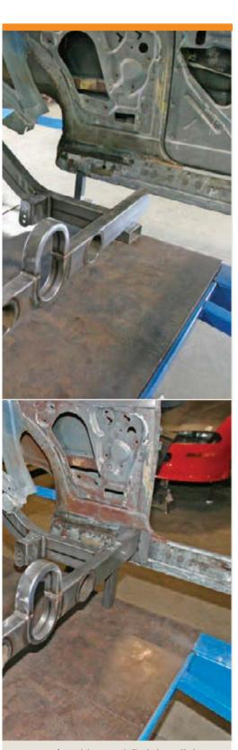
Bobby's satisfied that all the components are properly lined up and no binding occurs). Note the built-in driveshaft safety loop and 4-inch exhaust cutouts incorporated into the frame from Chris Alston's Chassisworks.
