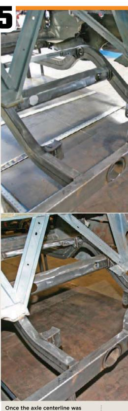
determined, the rear frame was mocked up under the Nova, measured for length, and trued to the vehicle itself. After the crossmember and the rear portion of the frame were cut, it was tack welded into place (the frame will be fully welded once
