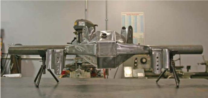
Pictured is the rear frame section from Chris Alston's Chassisworks all tacked in and ready to receive the FAB9 rear. Stay tuned for the next issue of Super Chevy as we show you how to properly narrow a 9-inch rear housing with the special tools needed to square the housing ends, weld 'em on, and garnish it with products from both Strange and Wilwood Engineering.
