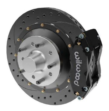
**Description:** g-Street front disc-brake for Chassisworks sculpted spindle. Minimum wheel diameter of 17" is required for use. Not for use with positive offset wheels.
