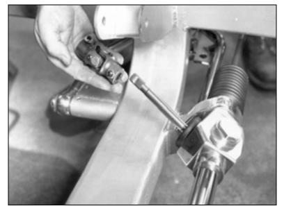
The first step in aligning the new A-arm front suspension is to center the rack in its travel. Placing a U-joint on the rack makes turning it easy.
