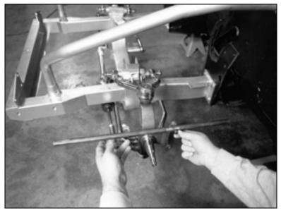
The adjustment for both caster and camber is made through the adjustable rod ends on the upper A-arms. Moving both rod ends out increases positive camber.
