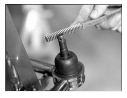
The balljoint castle nut will not thread on easily if the threads are nicked. A thread file can be used to correct the problem. After filing, try the castle nut again before putting the spindle on. Thread files can be found at most auto parts stores.
