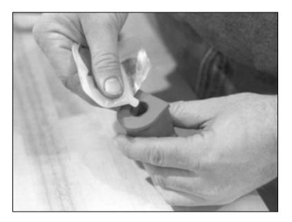
To prevent the urethane bushings from squeaking in action, use the supplied silicone grease to coat all sides of the urethane bushing that contact a metal surface. A thin screwdriver can be used to smear it around inside the bushing. Take extra care not to get this grease all over, it's very sticky.
