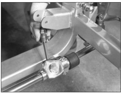
Turn the rack toward the passenger side of the car until it stops (full lock position).
