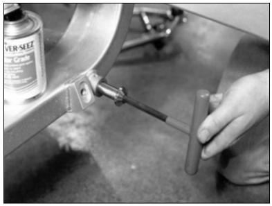
Now, apply some anti-seize to the threads of the pivot stud. Also put anti-seize inside the bore of the A-arm mounts. Insert one of the lower A-arm pivot studs and then run it in all the way to its stop, it should go in easy. Use the same procedure to verify all of the pivot studs will easily thread into their mounting locations.
