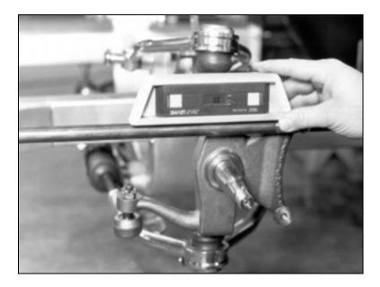
Next, set the bar level and tighten it down. Do this on both the driver and passenger sides.
