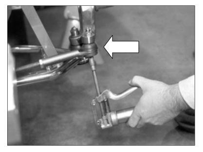
Grease the tie rod end with a small grease gun. Add only enough grease until a small amount starts to come out from under the rubber boot.
