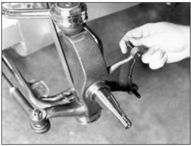
Next, check the caster by installing the 3/8-16 x 1 3/8" caliper mounting socket head allens (supplied in your brake kit) into the threaded bosses on the spindle.
