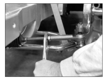
If rotating the tie rod end 360 degrees changes the toe-in too much, use the rack tie rod to make smaller adjustments. Put the tie rod end in the steering arm and snug the castle nut before adjusting. Use vise-grips to grab onto the tie rod and rotate it to adjust the length. Be careful to turn both tie rods the same amount.
