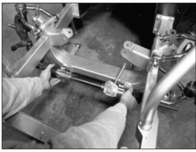
With the lower half of both rack mounts installed on the crossmember, the rack itself is set into position.
