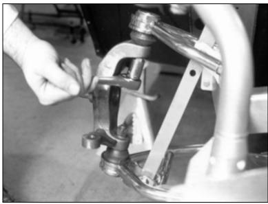
Repeat the procedure for the upper A-arm. First tightening the castle nut.
