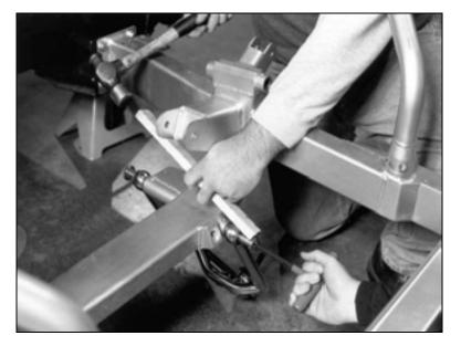
If you have to remove the lower A-arm pivot studs, use a piece of wood and a few taps with a hammer while turning the pivot stud counter-clockwise. The pivot stud will come out easily.
