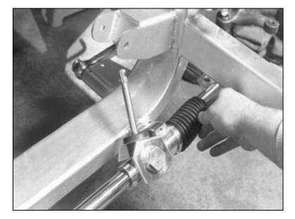
If additional clearance is needed between the pinion and the crossmember, you can raise the pinion up higher. A lower angle will be used to clear the side motor mount bracket. Rotate the rack to minimize the u-joint angle.
