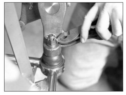
With the cotter pin installed, use pliers to fold the legs over the castle nut. One leg goes down the other over the top of the balljoint stud.
