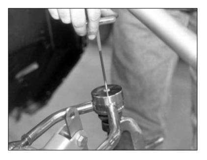
The caps are held in place with the countersunk stainless steel allen screws provided. They screw into the hole where the grease zerk was just removed. Be sure to remove all grease from the threads in the balljoint and Loctite™ the countersunk allen head screw in place.
