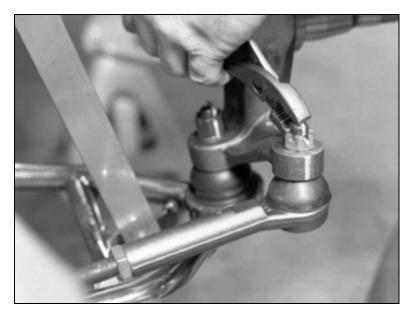
Put the tie rod ends back into the steering arm. Tighten the castle nut and, install and bend the cotter pin like you did on the balljoints.
