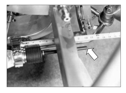
On the driver side, measure and record the distance from the rack mount to the end of the tie rod end. In our example the length is 9 3/4 inches.
