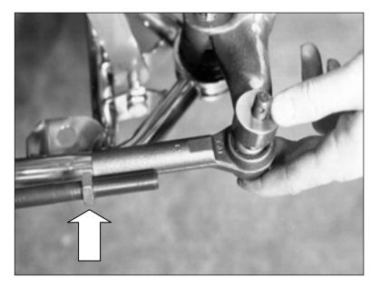
Install the tie rod end in the steering arm. Hold it in place next to the tie rod and adjust the jam nut until it is against the tie rod end.
