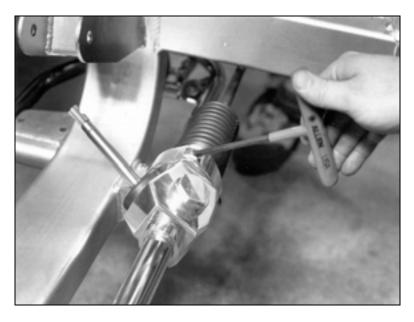
Tighten the cap with your T-Handle Allen wrench. Once you have the cap tight, the next step will be aligning the front end.
