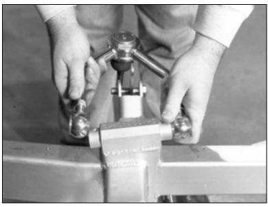
Installing the upper A-arm is similar to installing the lower A-arm. Slide the front rod end over the front mount first and then swivel the rear one into place.
