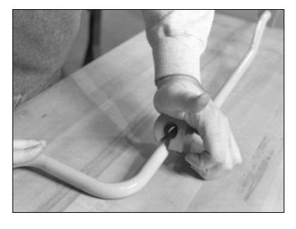
Once the slot in the bushing is opened, slide it over the antiroll bar near the 90-degree bend.
