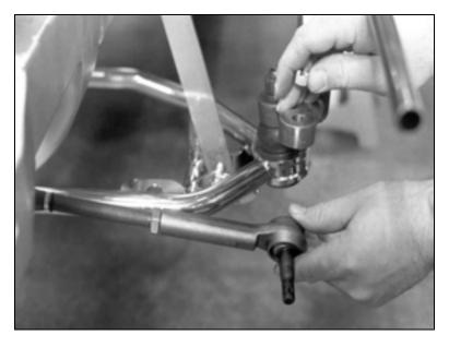
To adjust the toe-in, rotate the tie rod ends to move the spindle in or out as required. Make sure to rotate both the driver and passenger side the same amount. One-half revolution of both tie rod ends will change the toe-in by approximately ¼ inch, front to back.
