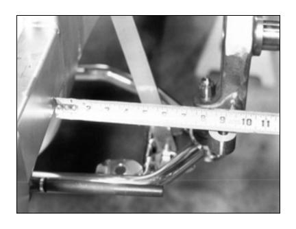
With the rack & pinion centered, you can set the spindle alignment. Measure from the outside of the frame to the inner edge of the tie rod hole in the steering arm. Set this dimension to 8 5/8 inches. This will make the spindle straight forward while you adjust the tie rod length.
