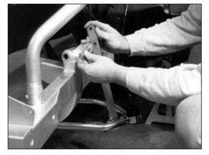
Next, install the shock simulator at the ride height position. Install the lower bolt first and then the upper.
