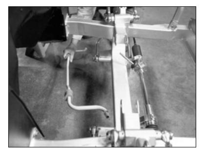
With both bushings on the bar, bring it up from under the car and set it in position.
