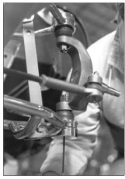
Use the same procedure to install the lower balljoint caps.
