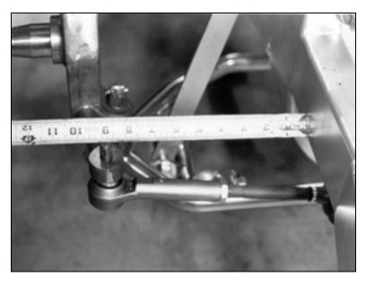
Repeat this procedure for the passenger side. The measurements are the same as the driver side.
