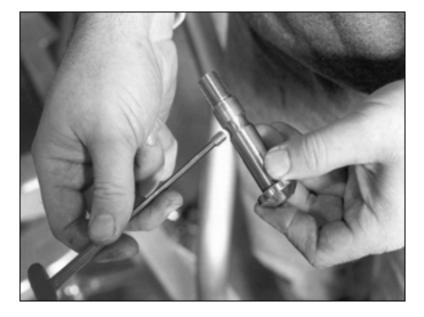
A set screw is used to lock the A-arm pivot studs. The set screw locks on the groove machined into the pivot stud.
