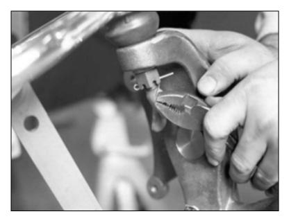
Install the cotter pin and fold the legs over as we did on the lower one. Repeat this procedure on the passenger side of the car.
