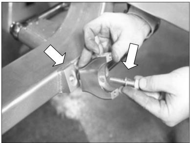
The rack-mounting bosses are factory welded to the frame. Use the  $1/2-13 \times 2$ " socket head allen and custom 1/2" lock washer to mount the lower half of the billet rack clamp to the mounting boss. Use a small amount of Loctite<sup>TM</sup> on the socket head allen.
