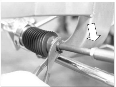
When turning the tie rods, the rubber boot will "wind up" on the tie rod. Once the toe-in is adjusted, use pliers to "unwind" the boot around the tie rod. Gently grab onto the outer boot clamp and twist it back around until the boots are straight. The jam nuts can now be tighten against the tie rod ends.
