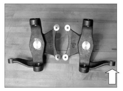
You are now going to install the dropped spindles. The "L" cast into the back of the spindles, does not designate "Left," it is the foundry mark. The best way to identify the driver and passenger side spindle is to remember the steering arm (shown with arrow) always goes toward the front of the car.
