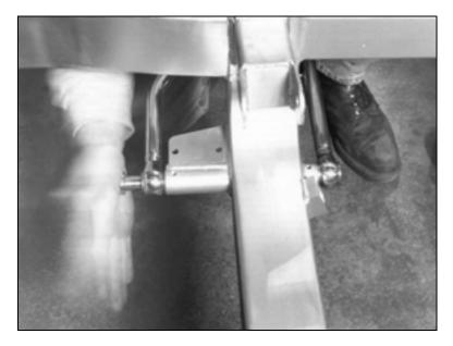
When installing the lower A-arm pivot studs, be careful not to damage the threads. Tap the pivot stud into place with your hand.
