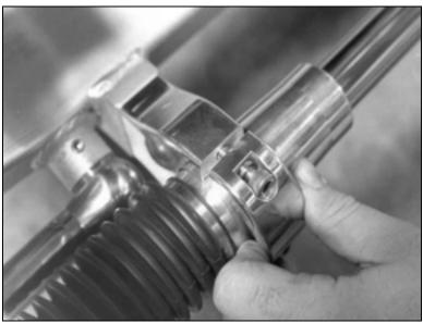
Push the rack firmly into each mount. Secure the rack by installing the billet rack clamp caps. Use the provided 5/16-18 x 1" stainless steel socket head allen and custom lock washer. Use a small amount of Loctite™ on the socket head allen.
