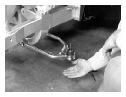
The lower A-arm should also stay suspended when released. It should take a few pounds of pressure to make it move.
