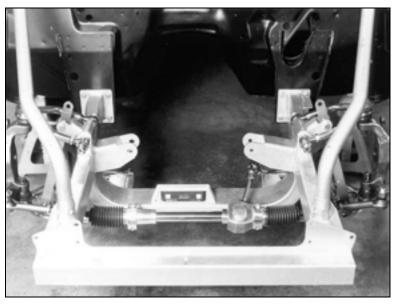
A readout from a digital level is preferred for accuracy when setting the front-end alignment. Level the crossmember and if needed, adjust the height by placing shims under one of the jack stands.
