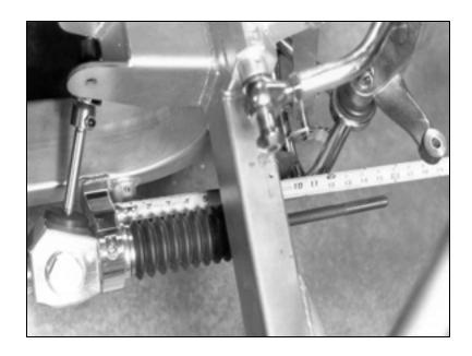
Next, turn the rack all the way to the driver side and record the measurement from the rack clamp to the end of the tie rod. In our example the length is 15 inches.
