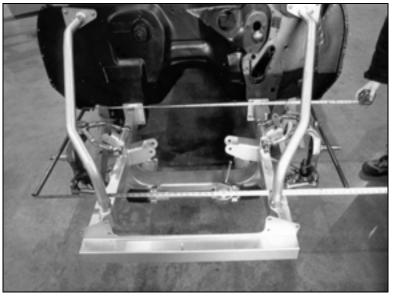
Using two tape measures, measure the outside width at the front and the rear of the tubes. The front dimension should be 1/8 to 3/16 less than the rear; this is the total amount of toe-in. Record the front and rear dimensions and calculate the amount of toe-in by subtracting the front measurement from the rear.
