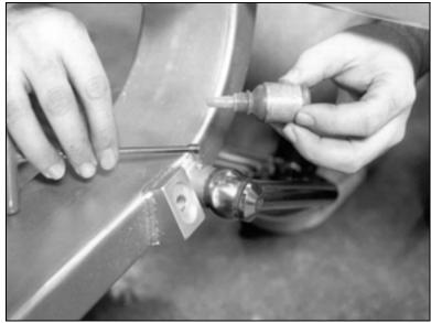
Before installing the pivot stud set screws, apply a drop of Loctite<sup>™</sup> thread sealing compound to the screws. Be careful not to get excess Loctite<sup>™</sup> in the pivot stud bore.
