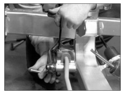
Slide the billet aluminum cap over the bushing and secure with the 3/8-16 x 2 1/2" socket head allen and locknuts provided.
