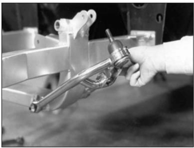
After tightening the lower A-arm pivot studs, check to be sure the A-arm swings freely but snugly throughout its travel.
