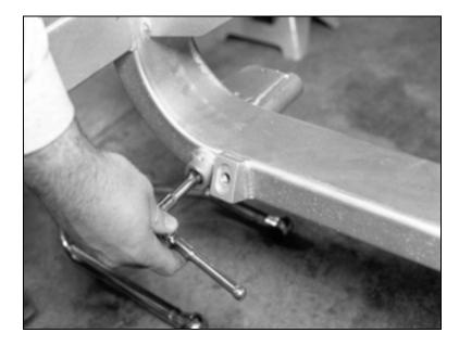
Next, chase the threads in the lower A-arm mounts with the 5/8-18 tap and blowout any remaining particles.
