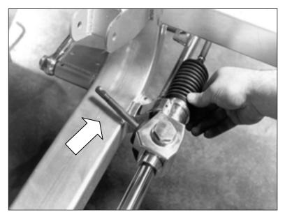
One of the exclusive design features of our rack and mount is the ability to rotate the rack to provide any desired angle from the steering column to the rack input shaft. Here the shaft is laid almost against the crossmember.
