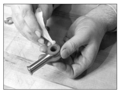
Coat the bushings with the silicone grease.
