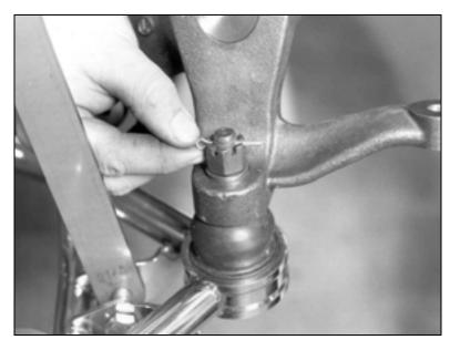
Insert the cotter pin through the hole in the balljoint. You may need to tightened it a small amount until the slots in the castle nut align with the hole.
