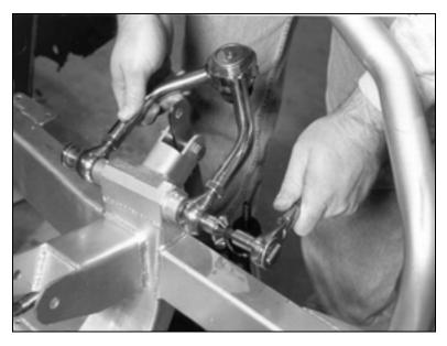
Install the upper mount bolts just like the lower mount bolts. Do not fully tighten them now because they need to be moved when we adjust the front suspension settings later. Repeat the installation of the upper A-arm on the passenger side.
