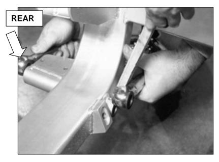
The lower A-arm fits tight over the mount. Slide the rear of the A-arm onto the mount and then use a piece of wood between the frame and the A-arm to pry it over the mount.
