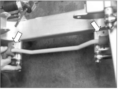
Center the bushings on the mounting pads welded to your frame.
