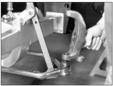
Place the driver side spindle over the balljoint and thread the 9/16-18 castle nut on.
