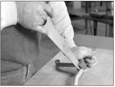
To open up the bushings, use the handle end of the balljoint wrench that is included in the suspension kit.
