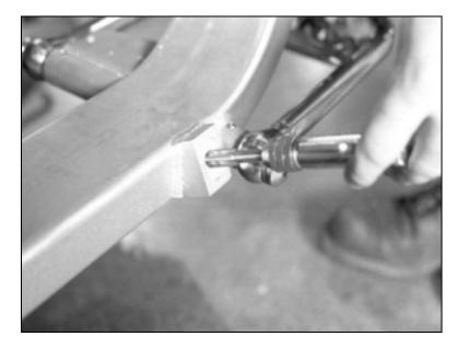
Mounting the steering rack is next. Chase the threads in the rack-mounting bosses with a 1/2-13 tap before mounting the billet mounts.
