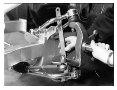
Loosely install the castle nut on the tie rod end. Make sure the spindle moves smoothly from full shock extension to full compression, as indicated by the holes in the shock simulator.
