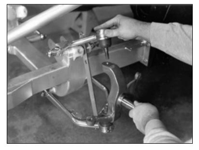
Place the spindle over the lower balljoint and install the washer and castle nut. The upper A-arm is then lowered into position and secured to the spindle with another washer and castle nut.
