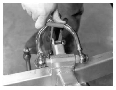
Once the camber, caster, and toe-in are set, tighten down the A-arm bolts and jam nuts, and install the set screws with a drop of Loctite<sup>TM</sup>.
