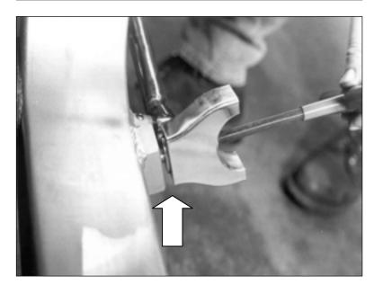
The raised section on the back of the billet clamp matches the milled recess on the mount bosses.
