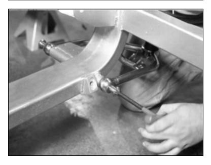
Once the pivot studs are in place, use an Allen T-wrench to tighten them. The pivot studs should go in easily and should be tightened until they are fully seated. This will give the bushings the proper amount of crush, and allow the lower A-arm to move with a small amount of resistance.
