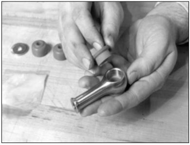
Put the urethane bushings into the upper antiroll-bar-link eyebolt.
