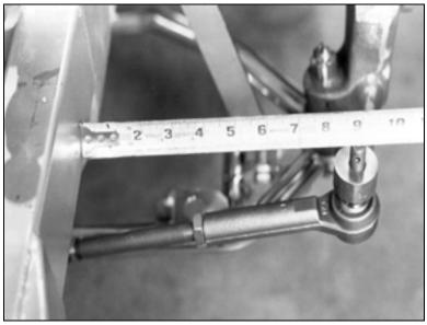
Remove the tie rod end from the steering arm and thread it onto the tie rod until it contacts the jam nut. Next, reinstall the tie rod end into the steering arm. Verify the distance from the frame to the inside of the tie rod end; this should be 8 5/8 inches as measured earlier.
