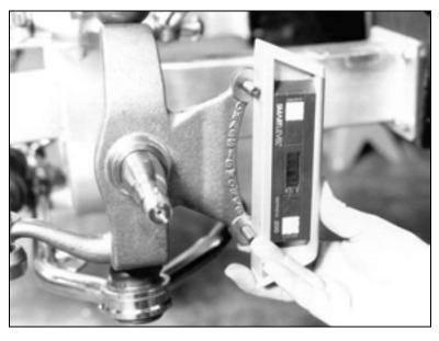
Set the digital level against the caliper mounting bolts. Record the caster reading. Positive caster is when the spindle top is tipped toward the rear of the car when viewed from the side.
