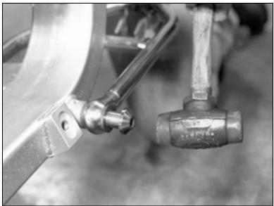
If the hand method does not work, you can use a plastic-tipped hammer to gently install the pivot stud. It is best to move the pivot stud a small amount at a time until the threads make contact.
