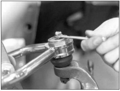
Grease the upper and lower balljoints. Install the zerk fittings and inject grease with a grease gun. Put only enough grease in to make the balljoint rubber boot bulge out on the side. If you are installing the balljoint caps, remove the zerk fitting.
