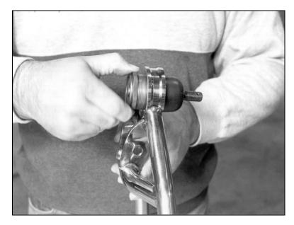
The balljoint is then screwed into the balljoint housing as far as possible by hand. Make absolutely sure that the thread starts straight. This is a little tricky. The threads on the balljoint are easy to cross thread.
