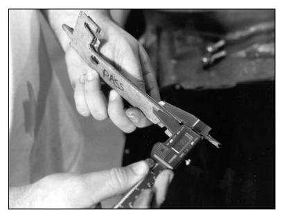
Next, get the stock shims for the passenger side and measure the thickness.
