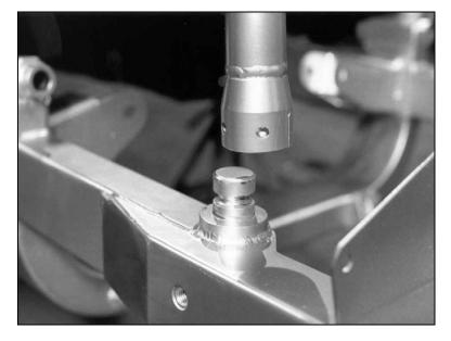
This is a close-up view of the Gemini connector. The female end, which is factory-welded to the strut, simply slips over the frame's male portion.
