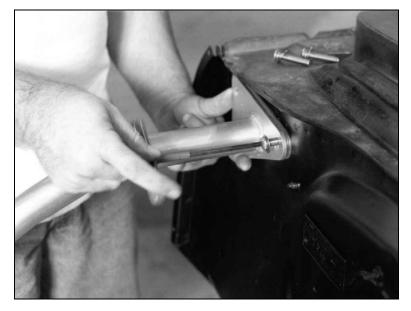
Use the 3/8-16 x 2" stainless steel button head allens provided to attach the upper strut plate to the firewall. Place the internal tooth lock washer on the button head allen first and then the flat washer. Do not fully tighten these until the driver's side is in place.
