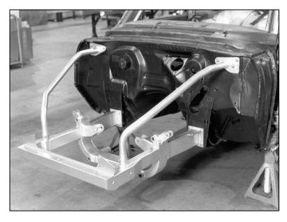
Place a floor jack under the subframe crossmember and raise it until the struts can be bolted on. You may need to raise one side more than the other. One person guiding the strut and a second person installing the bolts may help. After both struts are in place, tighten the lower mounting bolts, starting the four top ones first.
