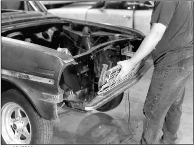
The grille, hood latch, lower pan, and mounting bracket can now be removed as one piece. There are seven bolts holding the assembly on. Two on the hood latch, two at the top front of the fenders, two below the splash pan near the radiator, and one on the lower core support crossmember. All of these fasteners will be reused. Put them in a bag labeled "grille bolts."
