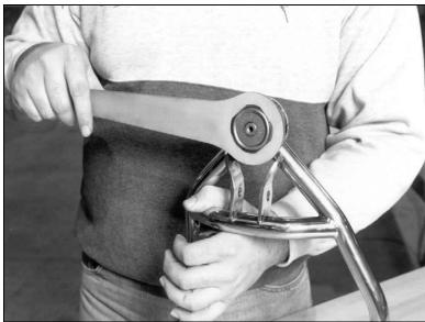
Use the balljoint wrench included with your kit to tighten the balljoint. Tighten it until it is fully seated against the balljoint housing. The force required can be over 150 lb-ft of torque. Be careful not to scratch the A-arm. Repeat this for the passenger side lower A-arm.
