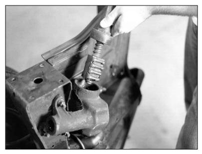
Pull the shaft free from the steering box and set it with the hood and fenders for later reuse.
