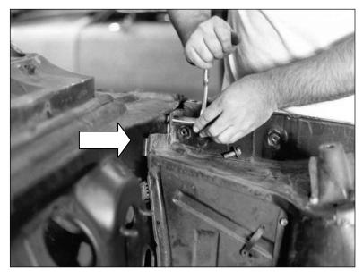
There are three bolts securing the top of the front clip to the firewall at each side. After removing these bolts, the shims between the frame and the firewall should slide out fairly easy.
