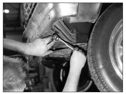
Next, drop down under the car and remove the bolts holding the bumper brackets to the frame. There are two on each side. There is no need to remove the bumper brackets from the bumper. Again, put these bolts in a bag labeled "bumper bolts."
