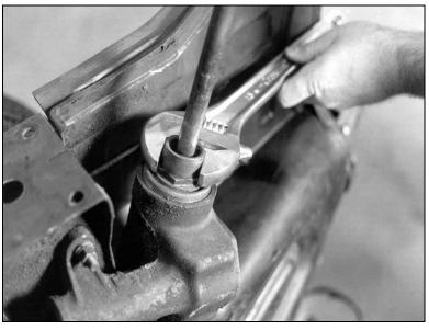
Unscrew the large nut holding the steering shaft itself into the steering box.
