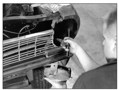
Remove all of the screws holding the headlight assembly in place. Once you have disconnected the wiring, bag the screws and set everything aside for later reuse. Use a bag labeled "headlight fasteners."
