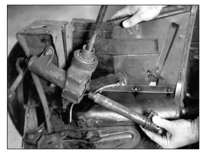
Slide the Pitman arm shaft all the way out of the steering box and discard it.
