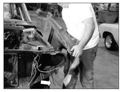
One bolt secures the lower front lip of the fender to a strut that is mounted to the radiator core support (visible between the fender and the tire). Another bolt holds the lower rear fender panel just in front of the door. Two more are found underneath the car. Remove these and the fender is free and ready to stack with the other parts.
