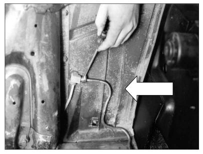
Disconnect the brake lines from the "T" fitting mounted to the inner fender panel. This is an inverted flare fitting. Using a brake line wrench works best to avoid damaging it.
