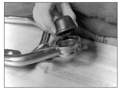
The balljoint rubber boot is installed in the balljoint housing first. Because the boot fits tight in the housing, installing it before the balljoint is easier. Drop the boot into the machined bore in the balljoint housing.
