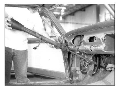
Now the column itself can be removed. Carefully pull it out. Watch to be sure all the wiring is free and it does not get caught on the brake and clutch pedals while removing.
