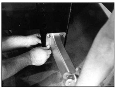
Attach the frame to the lower mounts using the 7/16-20 x 1 1/2 hex head cap screws, washers and locknuts provided. This is a high stress area, do not substitute other hardware. Once you have all the hex head cap screws installed, the front end will hang in place. Due to vehicle age, condition, and factory tolerances, the lower-mount angle will vary up to three degrees. Your new subframe will correct any variance.
