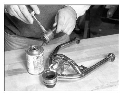
During the assembly process we are going to coat all of the threaded assemblies with an antiseize compound to prevent the threads from being damaged and aid disassembly in the future.
