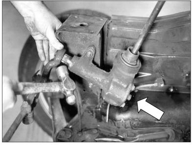
Once the nut is removed, a few taps of a hammer should pop the Pitman arm loose. If it is extremely tight, tapping on the side first will generally loosen it faster.
