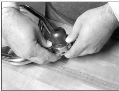
Work your way around the boot's edge, pushing it down into the bore with your fingers. You can also use a blunt tool to do this.
