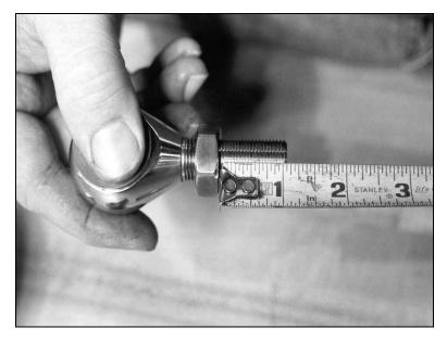
Install the rod ends into the upper A-arms. To provide an initial alignment baseline, the jam nut should be threaded until there is 1-1/16 inches of thread remaining past the jam nut.
