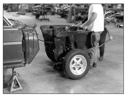
You are now ready to remove the clip from the car. Check to make sure all wiring and lines are disconnected.
