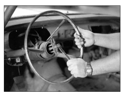
Next, remove the steering wheel and steering column from the car.
