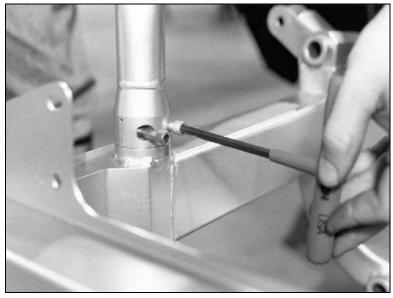
Two 5/16-24 x 1 1/4 socket head allens are installed to secure the strut to the frame. Do not torque these until we have the upper end attached to the firewall. These high strength alloy steel fasteners are highly stressed; do not substitute any other fastener.
