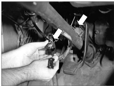
There are two electrical connectors that need to be unplugged. The first is the turn signal switch (shown in lower part of photo). The second is the neutral safety/back-up light switch (upper part of photo). Once unplugged, the steering column is ready to be removed.
