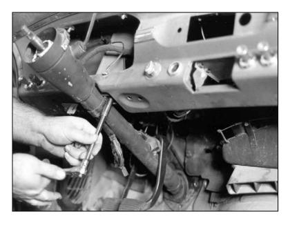
Next, remove the two bolts used to secure the steering column clamp to the underside of the dash. The column should now be loose.
