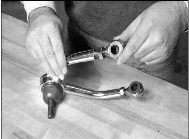
After the application of another dab of anti-seize, the rod ends are threaded into the A-arms, until the jam nuts are snug against the arm itself.
