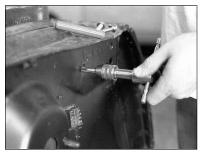
Before installing the upper strut plates, it is a good idea to chase the threads of the factory weld nuts. Make sure they are clear of any dirt or grime.
