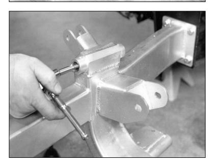
This step must be done carefully because the upper and lower A-arm mounts are threaded and welded to the frame. Use the 5/8-18 tap to chase the threads on the front and backsides of both upper mounts. Blow any remaining particles out of the hole with an air hose.
