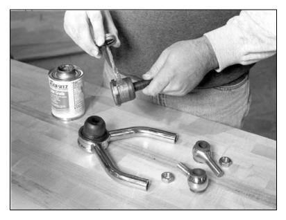
Next, apply a layer of anti-seize to the balljoint threads.
