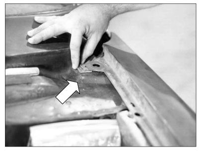
Now it's time to remove the outer fender panels. Remove the fender bolts and save the shims under the bolt located closest to the cowl on each side. Place these in a bag labeled "fender bolts."
