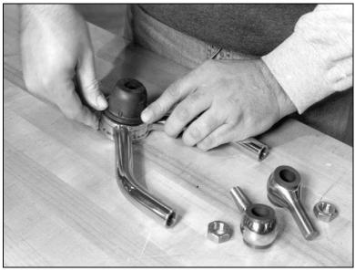
Use the same procedure to assemble the upper A-arm as the lower. First, install the balljoint boot into the balljoint housing.
