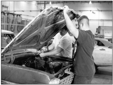
Now you will go to the outside and start by removing the hood. A second set of hands will make this easy. It is not important to mark the hinge location on the hood, because it will have to be realigned during reassembly. Once it is removed, set it aside. Put the bolts in a bag labeled "hood hinge bolts."
