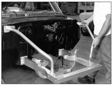
Repeat the process to install the driver's side strut. Once it is in place, tighten the inboard bolts at the firewall and all bolts on the Gemini connectors. Only snug up the outer bolts on the upper strut plate at the firewall until the hinge mount plates are installed.
