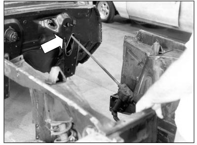
The steering shaft will remain with the nose of the car. Be careful when pulling the front clip away to avoid damaging the shaft, it will be reused with the new front suspension system.
