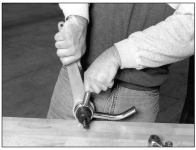
Finish tightening the balljoint with the balljoint wrench until it is seated tight against the balljoint housing. Repeat this for the passenger side upper A-arm.
