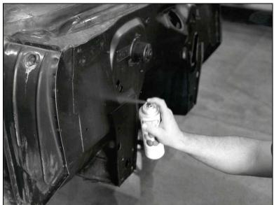
With the front end off, this is a good time to clean up and paint the car's firewall in preparation for installing the new front clip assembly.
