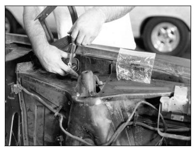
With the hood gone, it is time to remove the hinges. They are attached to the inner fender panel with two bolts on each side. Save these bolts in a bag labeled "hood hinge bolts" for use during reassembly.
