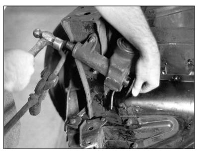
After removing the three bolts securing the back plate to the steering box, use a hammer to knock the Pitman arm shaft out. The shaft will rotate while it is being removed.
