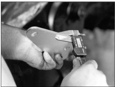
New shims are provided with the front frame kit; use as many as required (maximum of 4 per side) to achieve the same thickness as the factory shim pack measured. You may have to change the number of shims per side if the front fender-to-door gap cannot be adjusted to your satisfaction.
