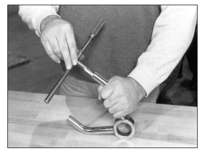
Use a 5/8-18 tap to chase the threads in the upper A-arm. Clear any debris left in the threads.
