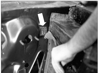
Unplug the electrical wiring harness at the firewall. Once it is unplugged you can remove the entire wiring harness from the front end, set it aside for use later.
