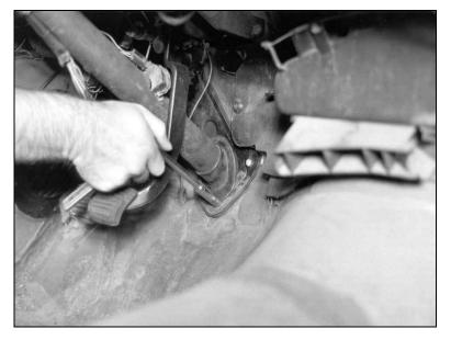
There are three bolts holding the lower column-mounting boot to the floor. Remove these bolts and place them in a bag labeled "steering column."
