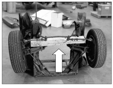
Here is the stock front end set nose-down on the shop floor, with the other pieces that have been removed in the background. The wood 4x4's suggested location is also clearly visible. This position facilitates the removal of the steering shaft.
