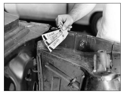
Label these shims to identify which side they were on, then place them in a bag labeled "front clip shims" and set aside. They will not be reused on your new Chassisworks front frame, but will be measured for total thickness and replaced with the custom shims included in the kit.
