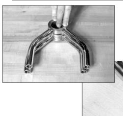
The upper A-arms will be assembled next. Although they are very similar, they are not identical. The letter "D" or "P" on the balljoint housing identifies which side of the car the A-arm installs in.
