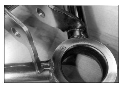
For identification, the driver side Aarm assembly is embossed with a "D" on the balljoint housing.
