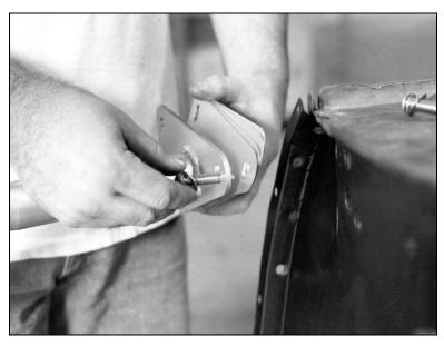
Take the appropriate number of new shims and install them on the backside of the strut mounting plate between the firewall and the plate. This will give you the correct alignment on the clip and the new upper hinge mount.
