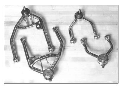
Installing Lower & Upper A-arms and Spindles
