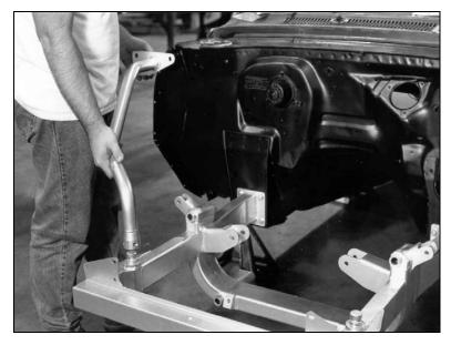
The next step is to install the front struts onto the male Gemini connectors that are factory-welded onto the frame.
