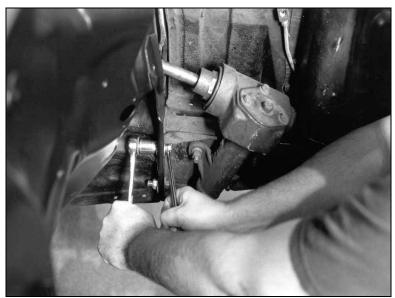
Removing the four bolts at the bottom of each side of the front clip is all that remains to separate the nose from the car. At this point, have an assistant on hand to keep the front end stable until you can get out of the way.
