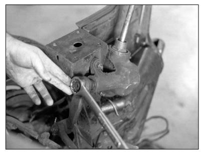
The steering box has to be disassembled to remove the steering shaft from the steering box.
