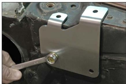
4. Using the bracket as a guide drill the three holes in the firewall with a 3/8" diameter drill bit. The two upper holes will go into the air vent box. The one on the face of the firewall goes through to the inside of the car.
