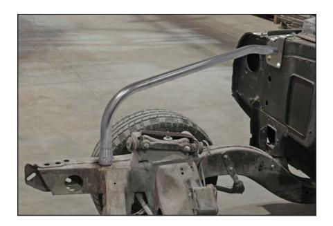
10. Once you have determined the location of the strut assembly on the subframe, use a disc sander with a scotch-brite pad to expose bare metal before welding.
