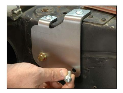
6. The alignment pin on the base of the joint plug is not used in this application and must be ground flush.
