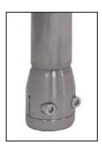
Position the strut assembly on the subframe and against the firewall plate as shown. The strut tube is purposely oversized so it can be trimmed to fit as needed. Adjustments to the length, angle, and height can be made by trimming the ends.
