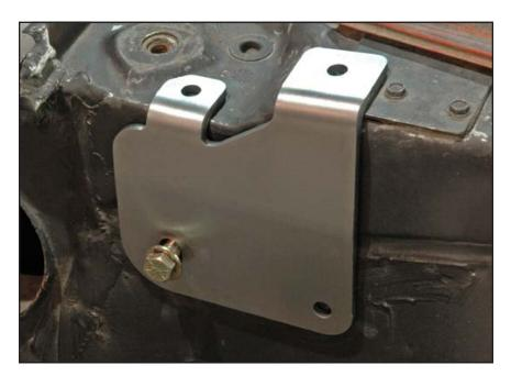
3. The bracket should be seated at the upper tabs and along the face of the firewall.
