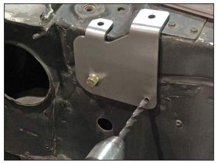
5. Secure the bracket to the firewall with the three 3/8-24 x 1" button head bolts, flat washers, and locknuts.
