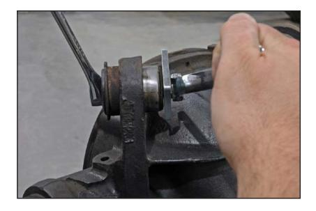
5. Use a hammer to drive the bushing toward the housing boss.
