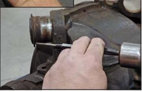
9. Once the bushing is removed, clean the inside surface of the bushing boss with a Scotch-brite pad before installing new bushings.
