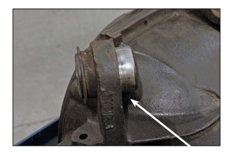
2. From the non-flanged side of the bushing, slide the 1/2-13 x 3" bolt through the slotted plate and then through the housing bushing sleeve.
