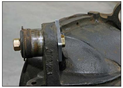
8. Use a flat punch to finish removing the bushing. Alternate tapping the on the flange at the top and then the bottom until it slides out of the housing boss.
