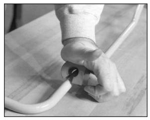
3. With both bushings on the bar, raise the anti-roll bar into position from underneath the car and set onto the welded mounting pads. Center the bushings between the mounting holes on each pad.
