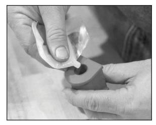
2. Use the handle end of the balljoint wrench to pry bushings open and slip over the anti-roll bar.
