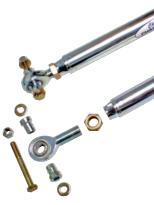
**Description:** Direct replacement 19-5/16" (center-to-center) length Pro Lower Control Arms, rod ends, jam nuts, reducer spacers, and mounting hardware. Fits 1982-1992 F-Body and 1978-1987 A & G-Body vehicles with 19-5/16" length factory lower control arms. **Note:** Not designed for use with factory rear anti-roll bars mounted at lower control arms.
