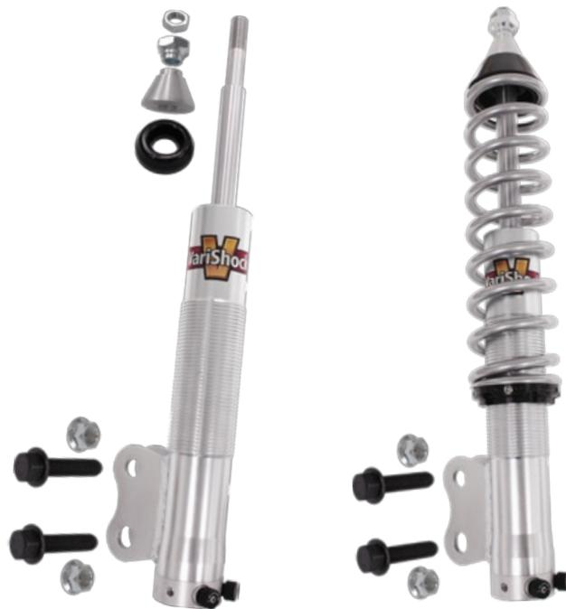
**Description:** Bolt-on strut directly replaces factory strut in 1982-1992 Camaro and can be used with coil spring in stock location. Additional components included with VAS 872DP-952 enable removal of factory positioned coil spring for conversion to 2-1/2" coil-over spring.
