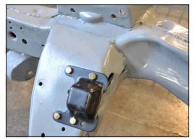
The new billet motor mount adapters will use the factory holes in the subframe. The driver-side adapter has the round hole for the billet mount. The passenger side adapter has a slotted hole.
