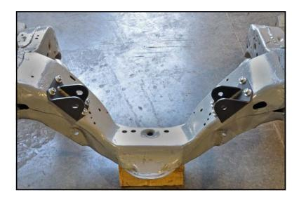
5. Once the billet motor mounts are attached to the engine they will slide into the adapters and be secured with the 1/2" hardware included with the mounts. Shown is the LS style billet mount.
