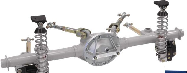
5829-A10 '64-67 A-BODY, DRAG RACE COIL-OVER SUSPENSION
