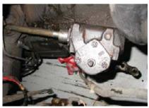
In order to get the steering box out of its home, the center link of the steering assembly needs to be unbolted from the Pitman arm. Once the column housing is out of the way, the box can slide out with the shaft.
