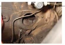
The Total Control rack kit comes with a new firewall pass-through bracket for the column. To remove the old one, unscrew the 3 Phillips-head bolts.
