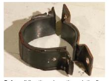
Before sliding the column through the firewall, we used the supplied adhesive pads on the factory clamp bracket. This is to keep the bracket from scratching our new Flaming River column.
