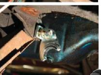
The Flaming River steering rack in the Total Control system uses the factory lower control arm mounting hole to mount its driver-side bracket. (There are three mounting brackets total: One for the driver's side, and two for the passenger side that consist of an inner and outer bracket.) The new supplied hardware should be snug, but not too tight to allow proper alignment with the other brackets.
