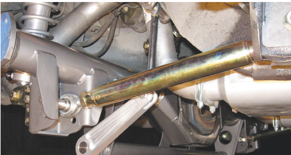
^ The Chassisworks Fab9 and suspension installation is complete, and now awaits a third member, axles, and brakes to round out the package. Keep your eyes on upcoming issues of Race Pages as we finish up the Panda's killer new rearend.
