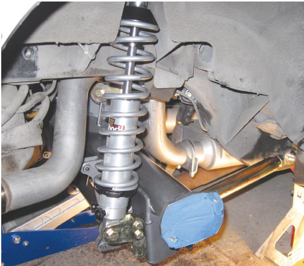
^ The coilovers install just like regular shocks, except that at the top, a spherical stem bearing takes the load instead of a polyurethane bushing. Because there's literally no friction on the bearing, it can be a challenge to feed the top stub through the hole in the mount up top, but it just takes a little patience. The shocks offer 16 'clicks' of independent adjustment in both compression and rebound, and Chassisworks can supply springs with rates ranging from 80 pounds per inch of compression all the way up to 450, with 175-200 typical for street use.
