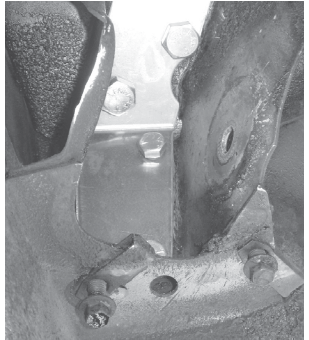
>> On Fox and SN-95 Mustangs, it isn't the control arm mount itself that fails; it's the connection between the stamped mount and the unibody that breaks. The stock mount and body are held together with a series of spot welds, and the kit from Wild Rides reinforces that connection by sandwiching it between two plates connected by four through-bolts. By spreading the load across a much greater expanse of unibody, the plates keep the stock mounts in place under duress.
