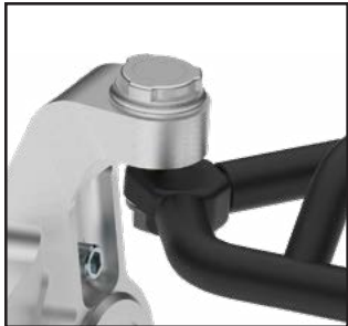
Upper Arm Pivot - Housed within the billet upright, the tension-adjustable pivot assembly can be tightened to compensate for wear.
