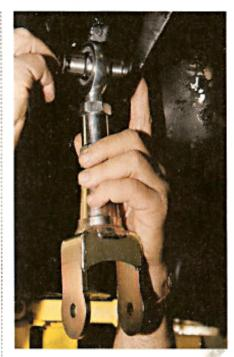
WE STARTED the FAB9 installation by installing both of the upper control arms onto the frame. Once they were on, we snugged them down but kept them movable to obviously link up with the housing later on.
