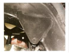
THIS IS the installed sway bar frame mount. Parsons welded the mount in the proper spot, then painted it black to match the rest of the underbody components.
