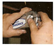
THE FAB9 rear we installed came with provisions to put in an antisway bar. We began by putting the sway bar mounts onto the housing. We had previously installed the sway bar, but we'll get into details of that a bit later. Keep in mind that each sway bar mount has to be indexed from side to side.
