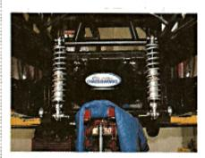
HERE'S A look at the back of the housing that shows the different position of the shocks due to the four-link design. You can see how the shocks are moved closer inboard, as opposed to the OEM mount position, which is further out on the axie tubes.
