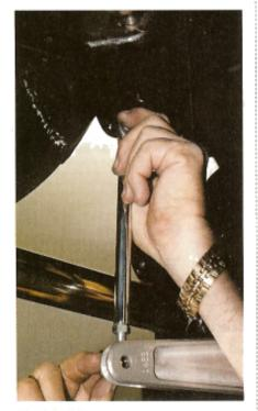
WE INSTALLED the sway bar links to the upper frame mounts.
