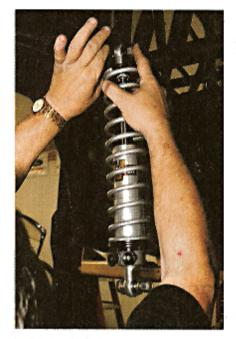
AFTER INSTALLING the upper control arms, we put in the shocks, mounting the tops of them to the proper point on the frame. As we did with the upper control arms, we left the shocks movable to link them up with the housing.
