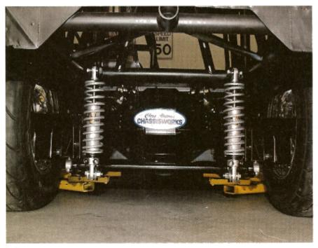
ONCE THE axles were in, the wheel and tire combo was bolted on, and the car was lowered to the ground. With no tinwork or anything else in the way, you can see just how good the FAB9 looks. We're sure it will perform well, too.
