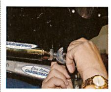
THE LOWER control arms were adjusted and hooked up to the housing. Once mated, the lowers were tightened, securing the car's rearend. Note: The control arm bushings are offset to allow for tire clearance.
