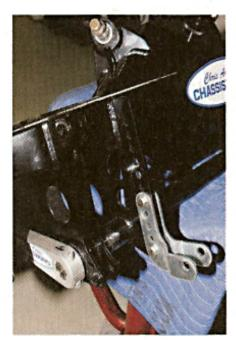
TO MAKE room for larger meats, the mounts for the shocks were moved inboard in relation to the factory shock mounts. The mounts for the coilovers are seen here with the supplied aluminum bracket already attached.
