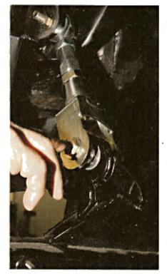
WE USED a transmission jack to raise the housing into the proper spot. Once the housing was in the car, we linked it to the upper control arms and tightened them down.
