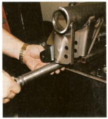
BEFORE PUTTING the housing into the car, we had the sway bar installed in the sway bar mount on the housing. This is a two-person job that is much easier to do on a bench than in the car. You slide the tube in from one end and finagle it to the other side.
