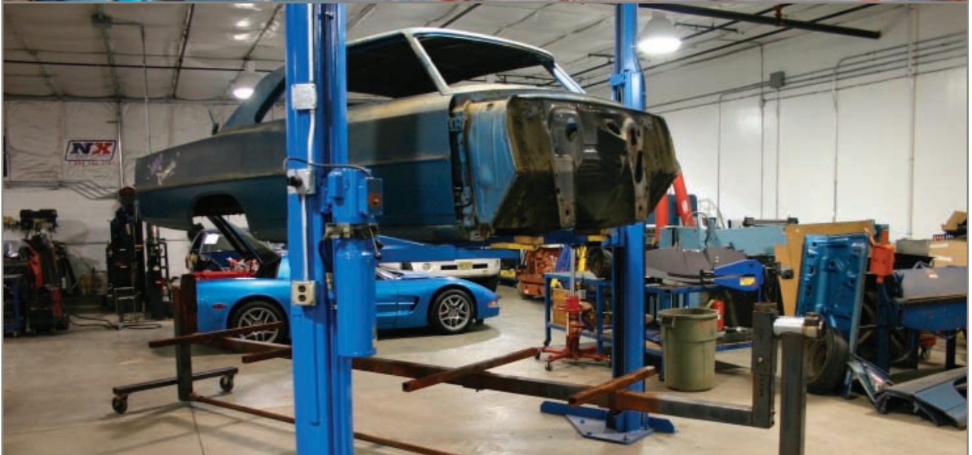
Eddie proceeded by stripping the interior of its gauges and all creature comforts. After completely stripping the Nova, it was mounted to the rotisserie in order to be blasted with some baking soda. Did that sound right?
