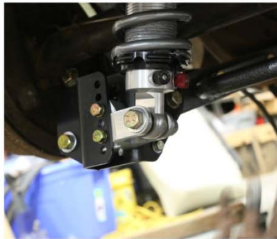
Each shock was bolted onto the lower mount, the bolts just snugged up.
