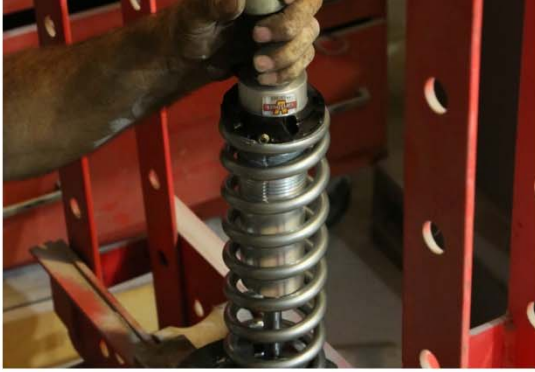
The springs for our car were quite stiff, so much so we had to use a press to get the upper spring keeper in place.
