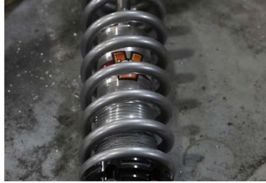
The assembled shock was left with the ring collars at the bottom of the threads. This will be adjusted on the car.
