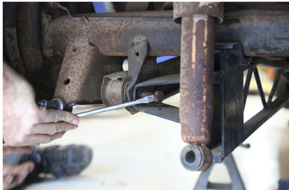
The lower trailing arms were also unbolted, along with the shocks.
