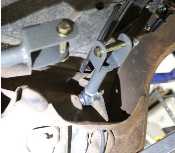
We also installed the upper control arms. All the bolts were loose, they didn't get torqued until the install was finished and the weight of the car was on the suspension.
