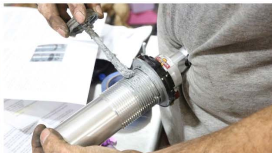
We coated the threads on the shocks with anti-seize. This keeps the ring collars from galling up on the aluminum shock body. Leave it off and you may very well ruin the shock.
