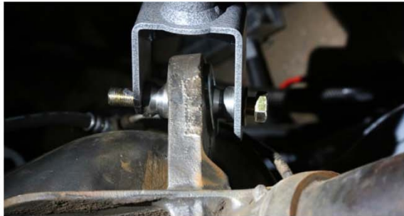
Up top, the articulating bearing makes for a much smoother ride, this allows for better travel and limits side to side deflection.
