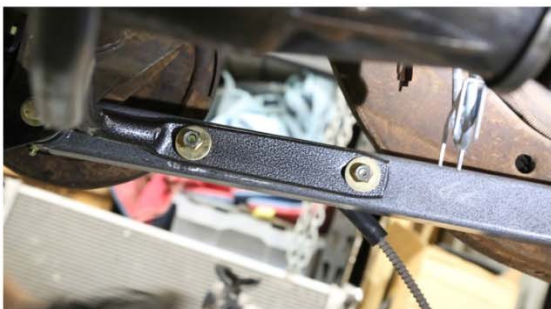
You will notice that the powder coating did get chipped a little during the process. It will be touched up with gray paint.
