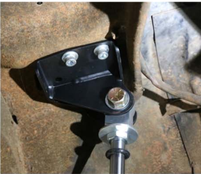
The upper shock mount requires drilling specific holes on specific year model vehicles. The mounts bolt in place with a couple of bolts and then the others are drilled accordingly.
