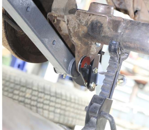
The housing was then bolted to the new lower trailing arms using the supplied washers.
