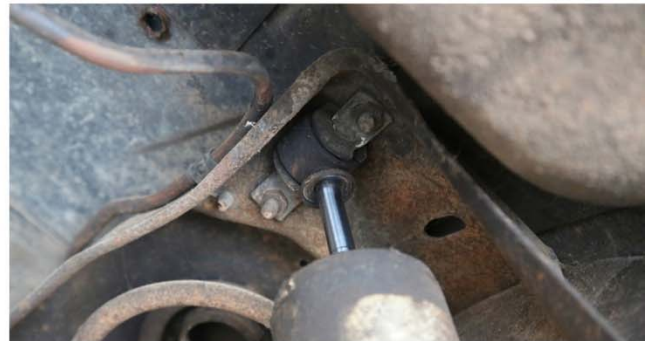
The upper shock mounts are next to the coil springs, you need a socket on the nut and a wrench on the bolt at the top. Be sure to use lots of lubricant on these old crusty fasteners.
