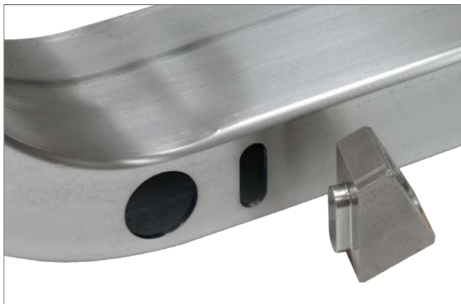
Billet rack-and-pinion mount inserts into machined slot on crossmember.
