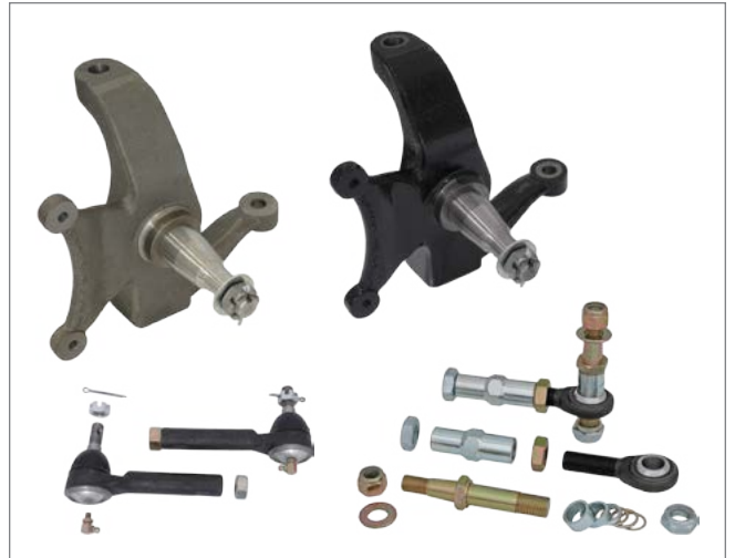
Spindle/Tie Rod Options: Sculpted spindle (bare, black) / OEM-style or bump steer
