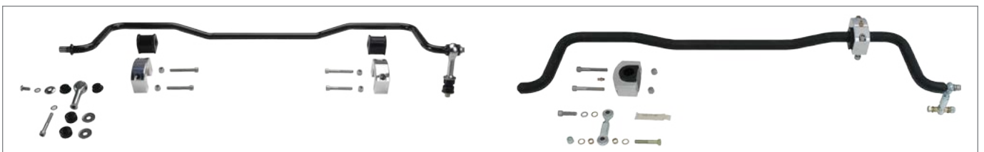
Anti-Roll Bar Options: Street Machine (3/4" solid bar with poly endlinks), g-Machine (1" or 1-1/4" tubular bar with bearing endlinks)
