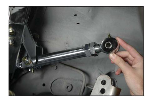
57. Bolt opposite end of each upper link to the lower hole at the axle bracket. Grease zerk must point up.
