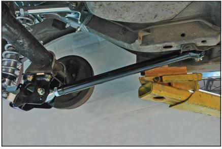
55. Adjust upper suspension links to 9-1/2" center to center of the mounting holes.
