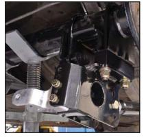
Shock Extenders (P/N: 300-0163 or 300-0164) Use with bolt-on or weld-on brackets.
