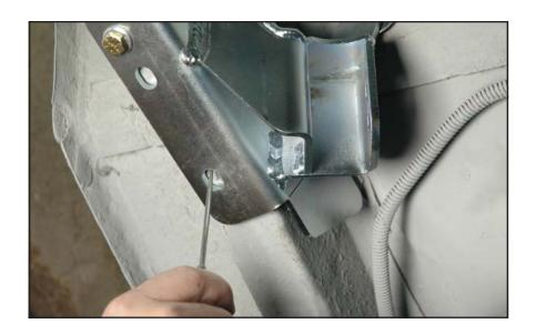
24. Use a 3/8"-diameter bit to drill a starting hole through the factory frame rail at each of the eight oval holes along the bottom of the frame rail ONLY. These holes will be opened up in a later step. The clamped cradle brackets will help to correctly guide the drill.
