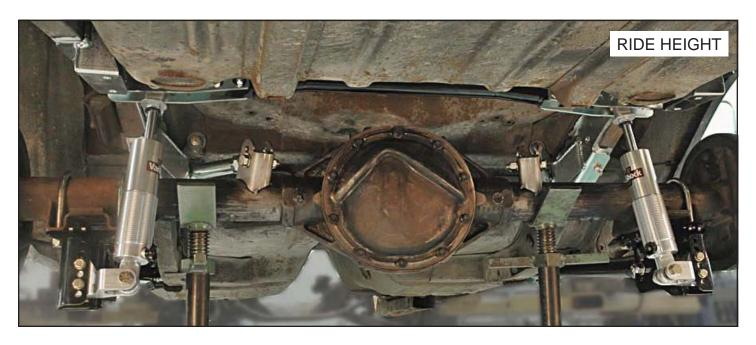
72. Using a jack, cycle the rear suspension through its full range of vertical travel and body roll in both directions to check for binding and potential clearance issues at all suspension joints and along the lengths of any moving parts including the rearend housing.
