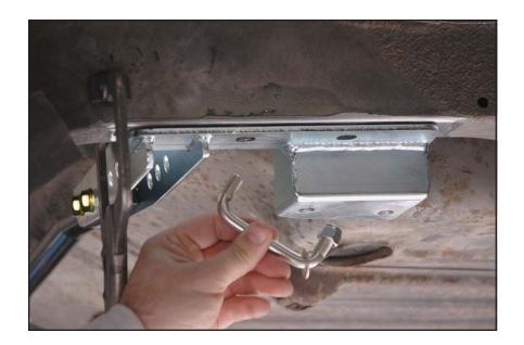
37. Slide the other end of the u-bolt into the hole in the frame brackets closest to the rear of the car, out through the second hole as shown, and secure with a flat washer and locknut.
