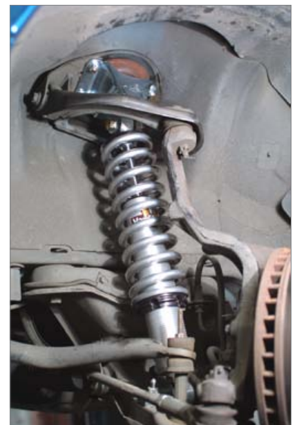
Coil-over kit includes springs, direct-fit upper shock mount and lower crossbar, upper spring seat, threaded locking lower spring collar, and mounting hardware.
